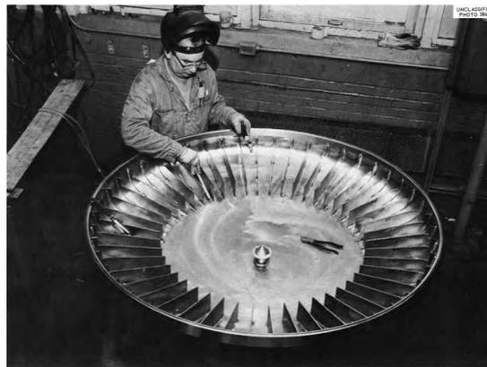
Figure 11: Assembly of Anti-Swirl Vanes and Drain Line in the Lower Head [42]
