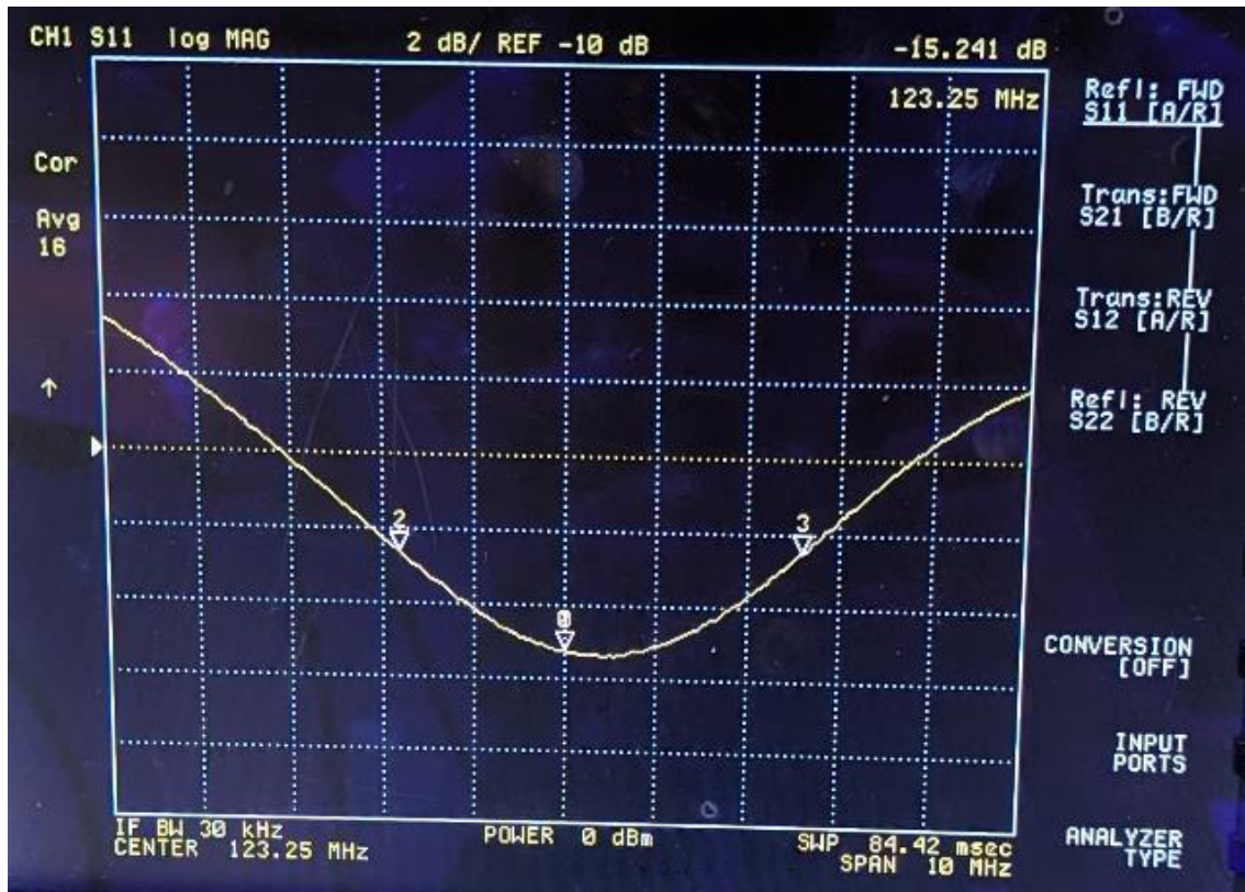
Fig. 3-10: A sample S 11 measurement of the 8-channel parallel radiofrequency coil with markers set for a quality factor calculation.
