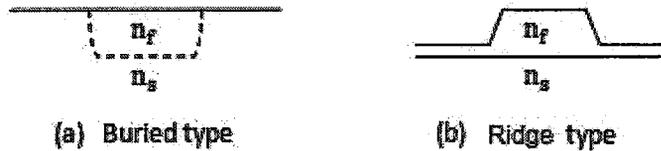
Fig.2.9 Typical structures of optical channel waveguides: a) buried type, b) ridge type. ( $n_f > n_s$ )
