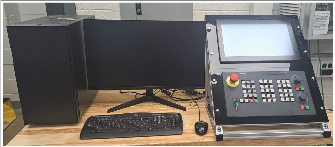
(a) HMI and computer with Siemens control software
