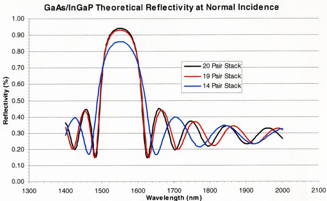
**Figure 5.2.4:** Theoretical Reflectivity of GaAs/InGaP DBR stack with various numbers of pairs at normal incidence.
