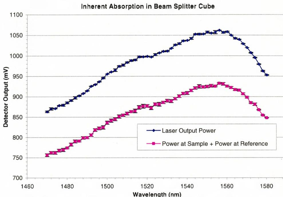
**Figure 2.3.6:** The two curves clearly reveal the presence of some type of loss in the beam splitter.
