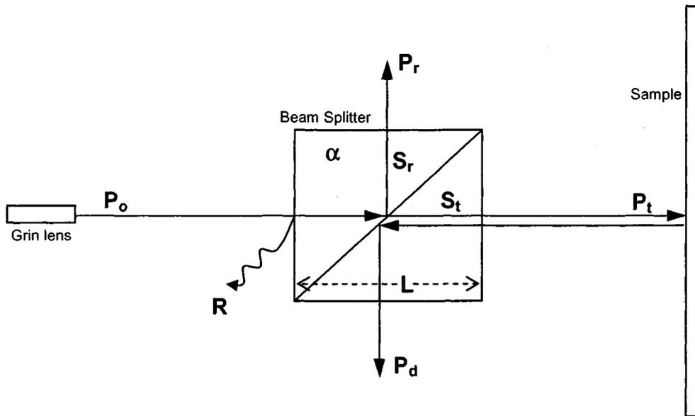
**Figure 2.3.7:** Illustration of variable assignments to beam splitter model.
