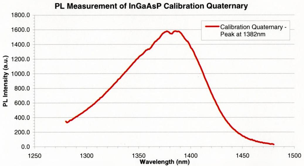
**Figure 4.7.1:** PL measurements taken for calibration purposes from a InGaAsP quaternary with identical composition as found in DBR stack.
