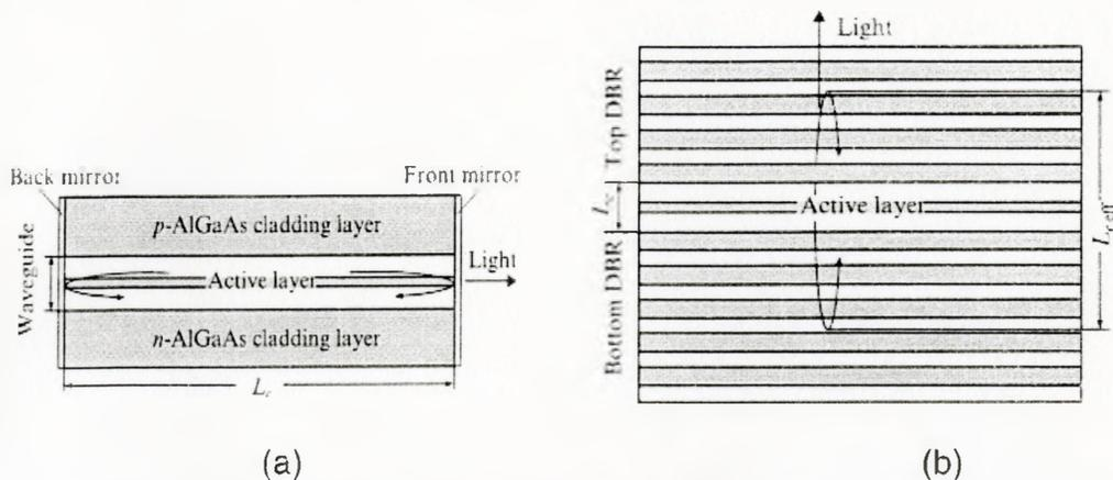
**Figure 1.1.1:** Cross-sectional diagram of a) edge emitting laser with large gain medium b) VCSEL with small gain medium [4].
