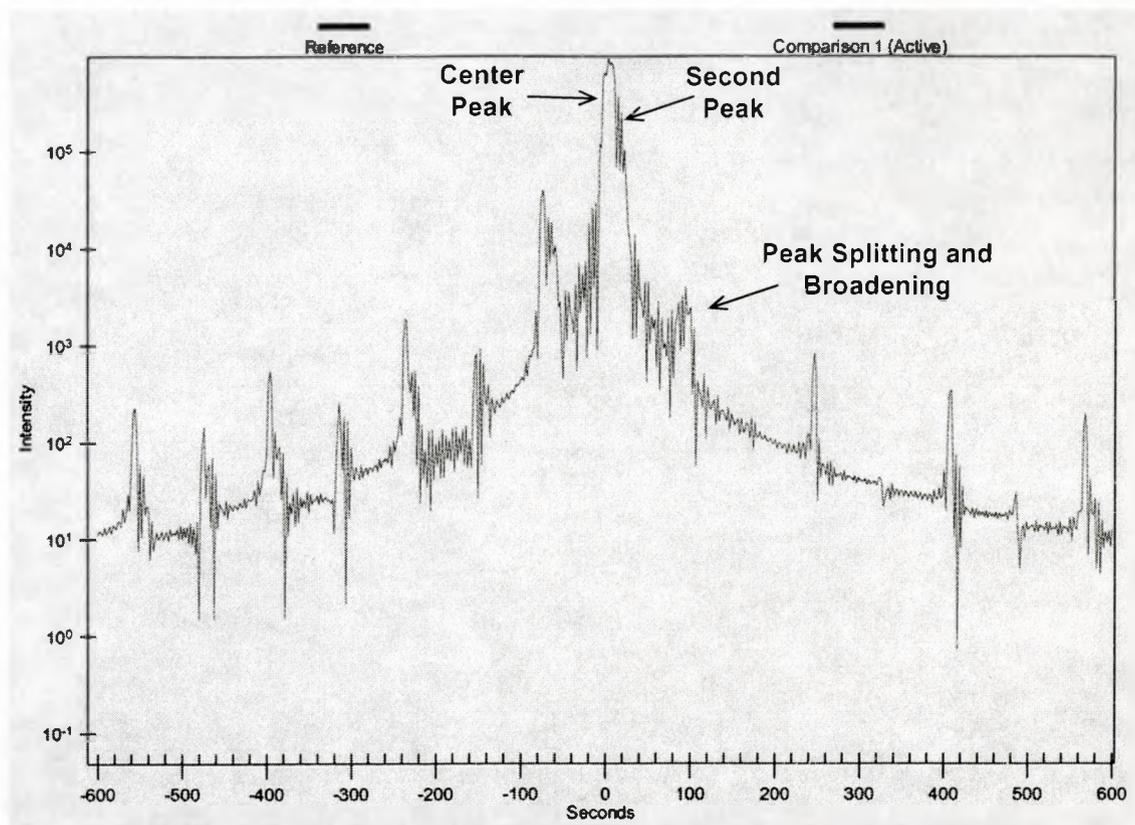
**Figure 5.4.4:** X-ray simulation of the 20 pair GaAs/InGaP DBR stack with a slight compositional change using Bede Version 3.0 software.
