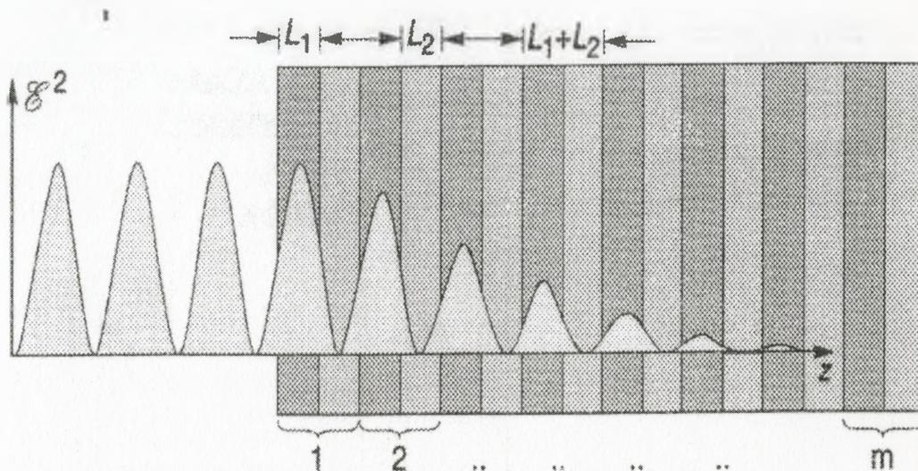
Figure 3.1.2: Illustration of the DBR penetration depth consisting of two materials of thickness  $L_1$  and  $L_2$  [3].
