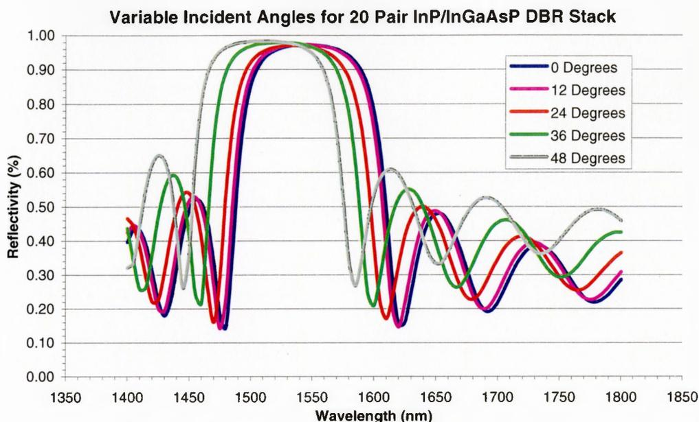
**Figure 4.2.5:** Variable incident reflectivity measurement of 20 pair InP/InGaAsP DBR stack.
