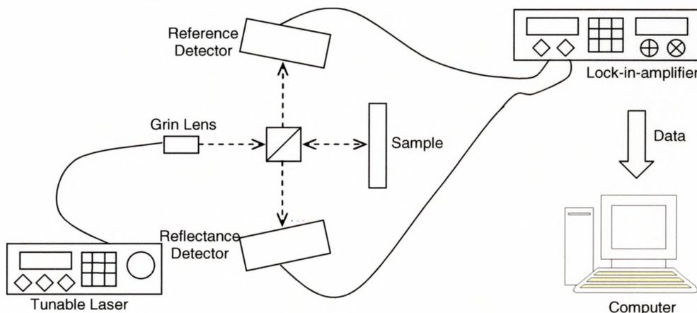
**Figure 2.3.1:** Normal incidence experimental setup.
