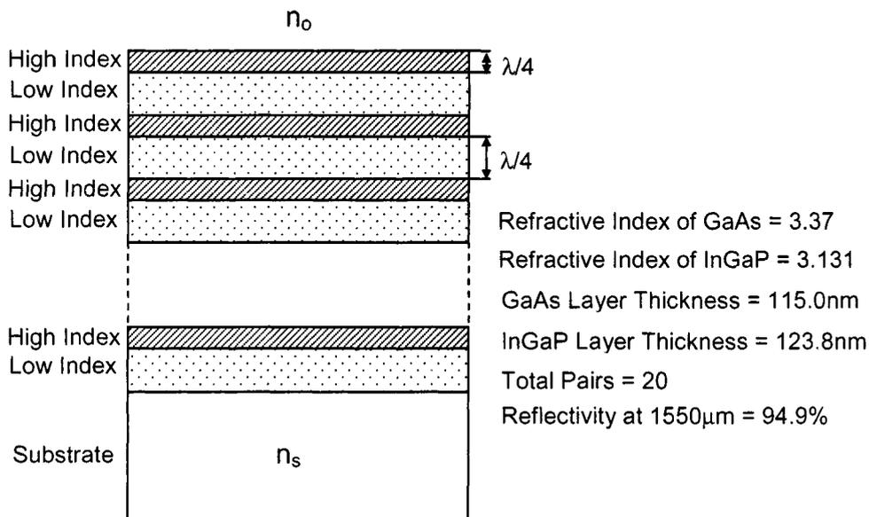
**Figure 3.6.2:** DBR design summary for GaAs substrate.
