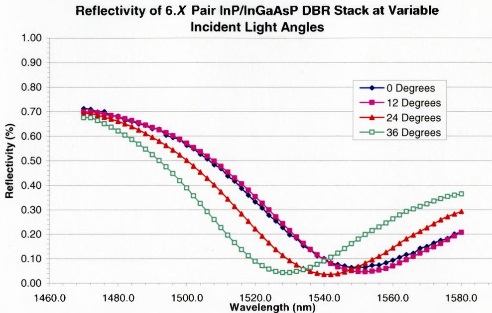
**Figure 4.4.1:** Plot of improperly etched 6 pair DBR stack resulting in alterations of reflectivity characteristics.
