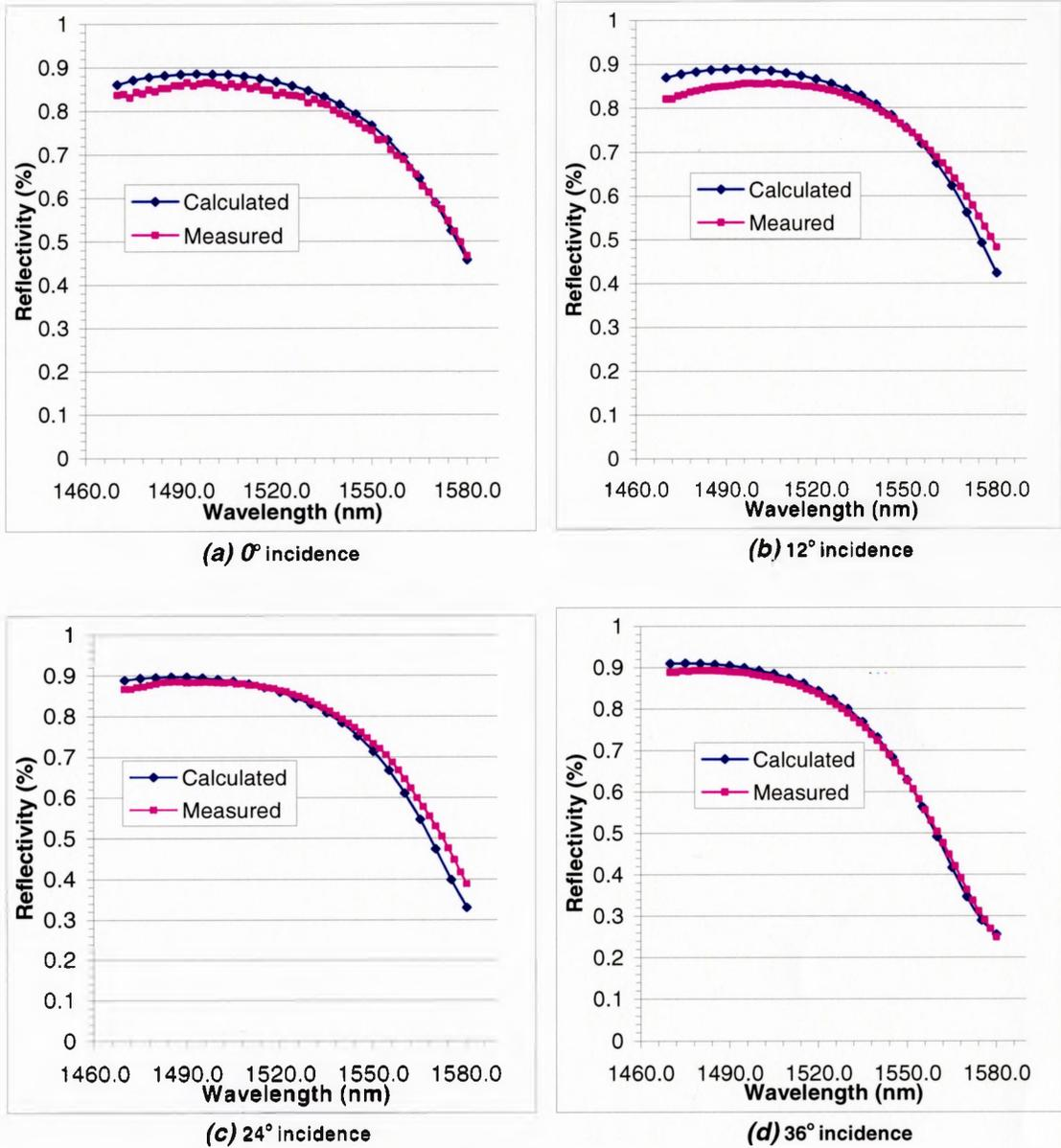
**Figure 4.3.5:** Theoretical fit to experimental data of 12 pair InP/InGaAsP DBR stack.
