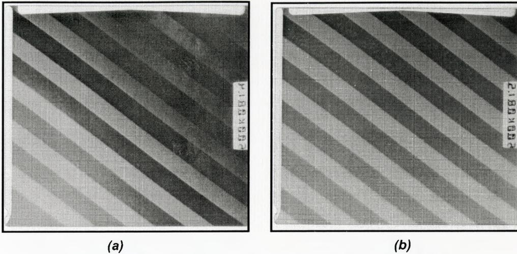
**Figure 4.5.2:** TEM micrographs of (a) bottom dozen layers and (b) top dozen layers of InP/InGaAsP DBR stack.
