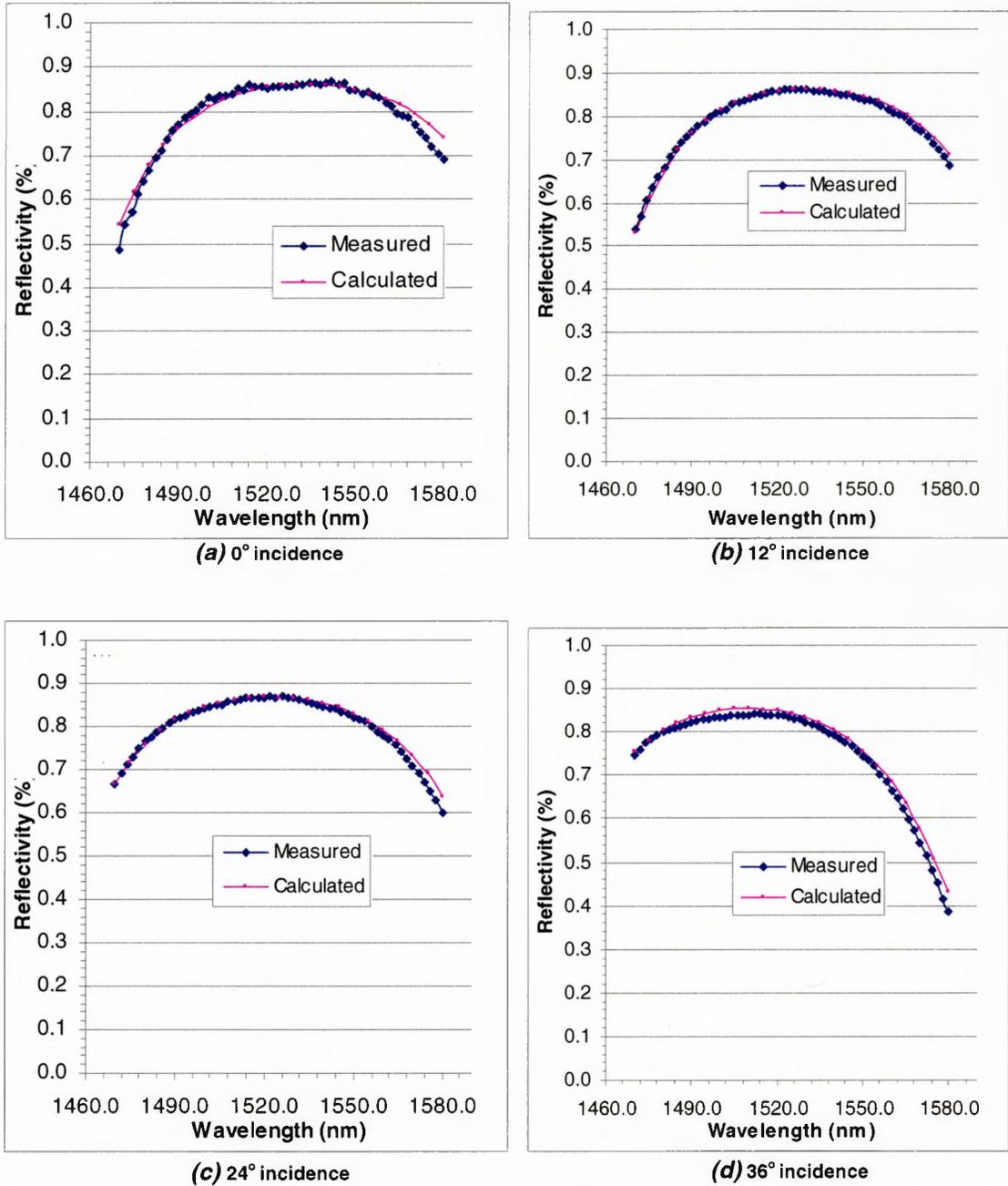
**Figure 5.3.3:** Theoretical fit to experimental data of 14 pair GaAs/InGaP DBR stack.
