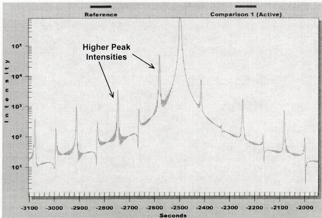
Figure 4.6.5: X-ray simulation of a 20 pair InP/InGaAsP DBR stack with a slight thickness change using Bede Version 3.0 software.
