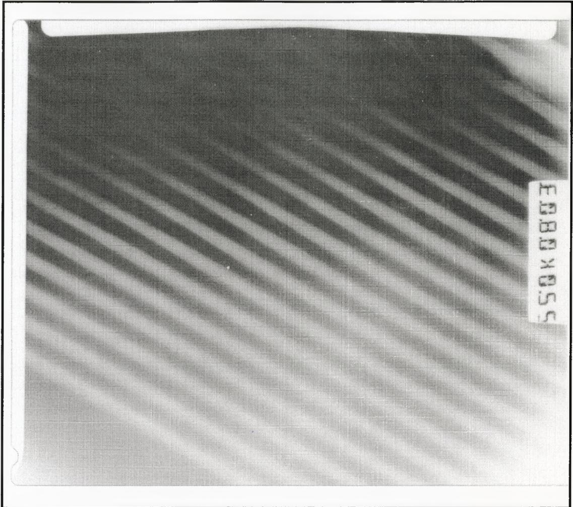
**Figure 4.5.1:** TEM micrograph of all 40 layers of the InP/InGaAsP super-lattice structure.
