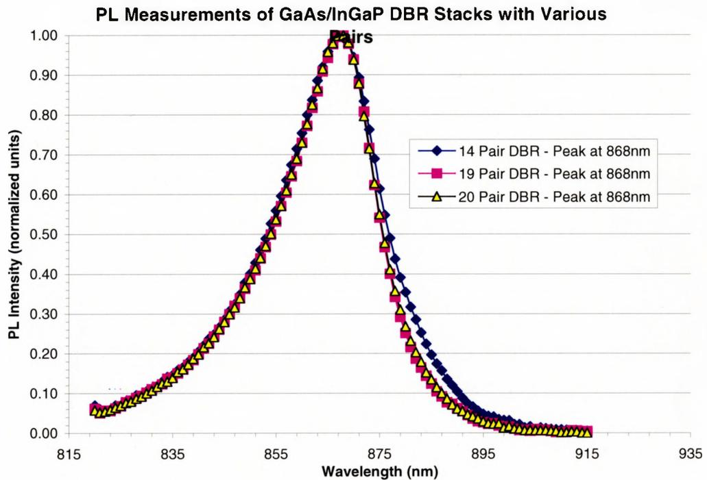
**Figure 5.5.1:** PL measurements taken from three GaAs/InGaP DBR stacks with various numbers of layers.
