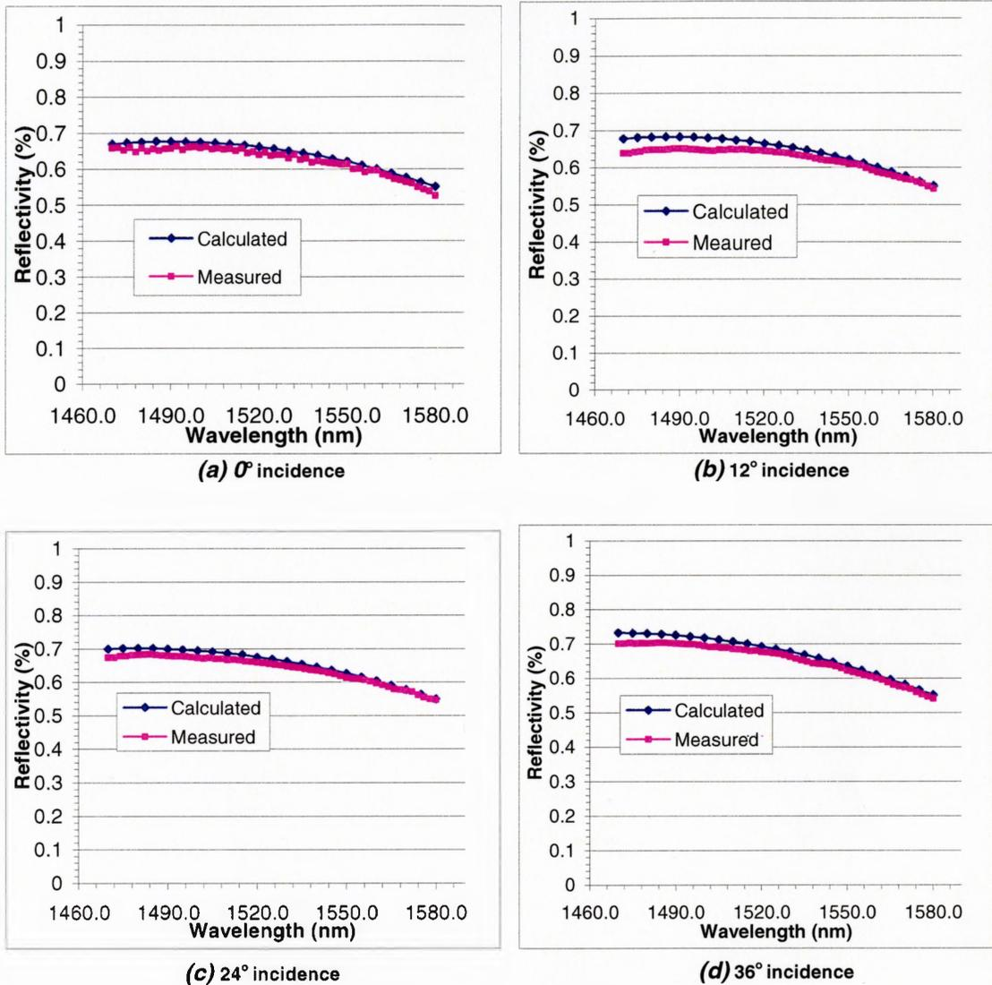
**Figure 4.3.6:** Theoretical fit to experimental data of 6 pair InP/InGaAsP DBR stack.
