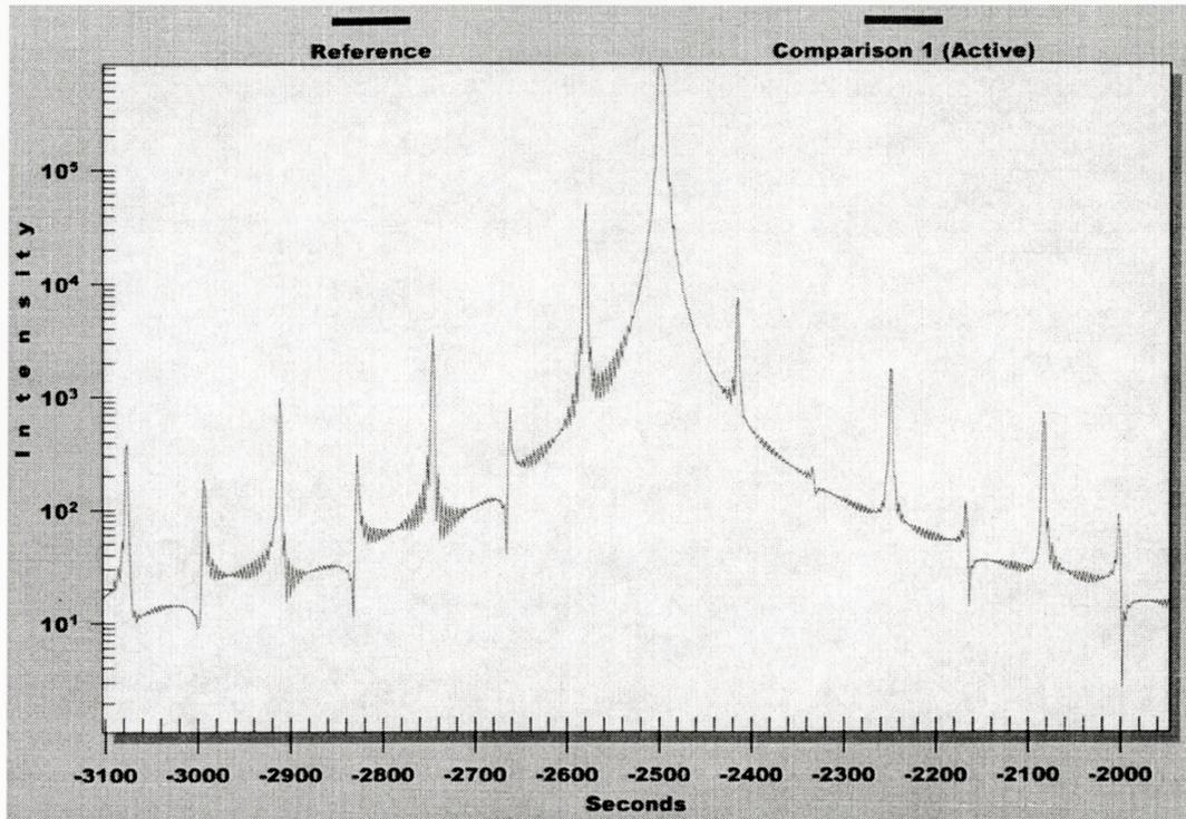
**Figure 4.6.3:** X-ray simulation of a 20 pair InP/InGaAsP DBR stack using Bede Version 3.0 software.
