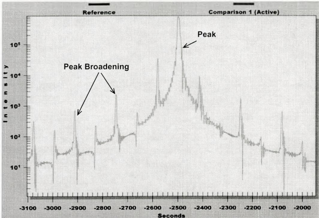
Figure 4.6.4: X-ray simulation of a 20 pair InP/InGaAsP DBR stack with a slight compositional change using Bede Version 3.0 software.
