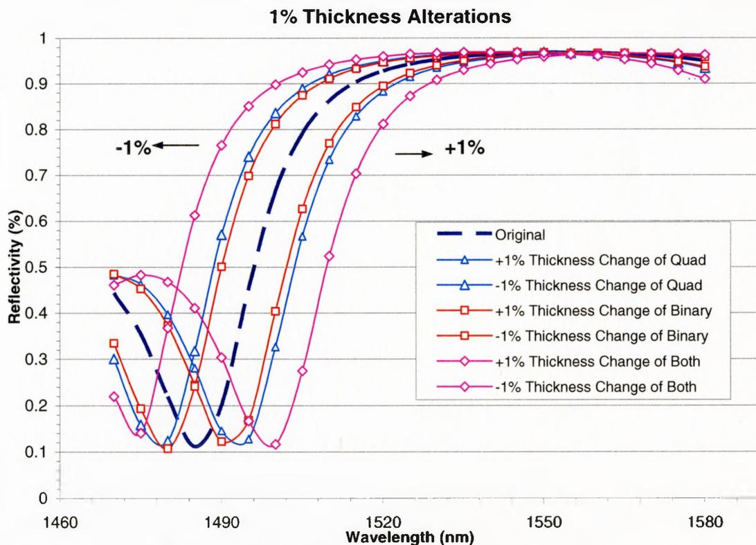
**Figure 4.3.1(a):** Observed effects of a  $\pm 1\%$  alteration in 20 pair DBR stack layer thickness.
