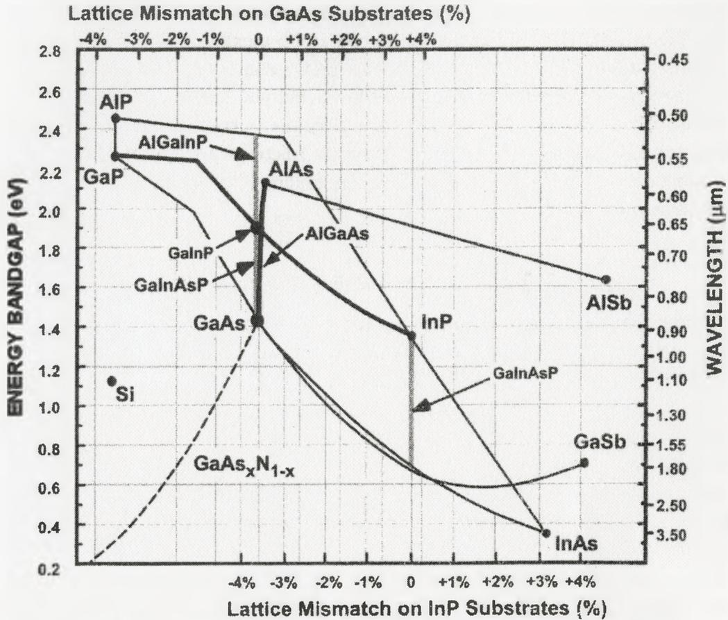
Figure 3.2.1: A plot of the dependence of band gap energy (emission wavelength) on lattice mismatch relative to GaAs and InP substrates [3].
