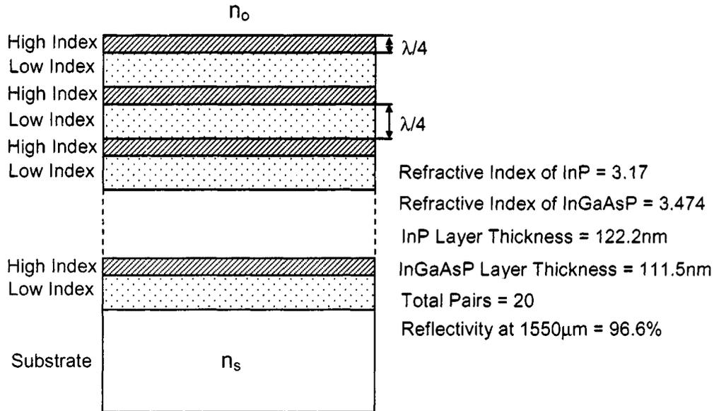
**Figure 3.6.1:** DBR design summary for InP substrate.
