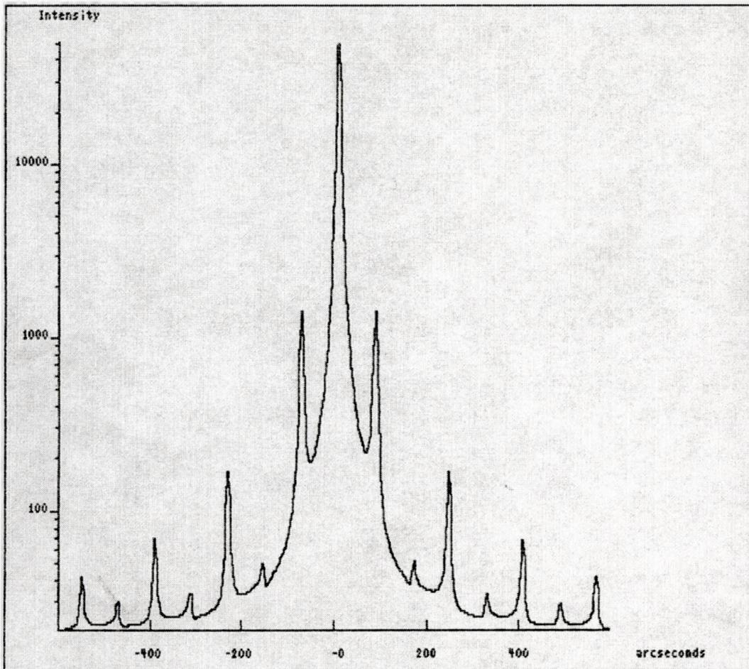
**Figure 4.6.2:** X-ray simulation of 20 pair InP/InGaAsP DBR stack using Bede original software.
