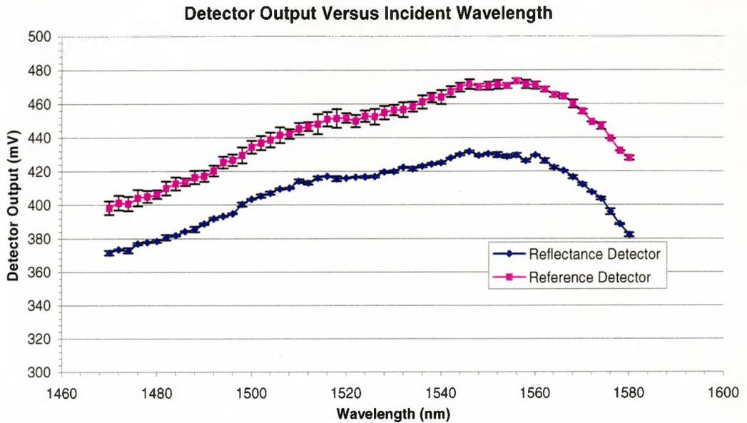
**Figure 2.3.3:** Typical wavelength dependence of both detectors shown for a fixed laser output power of 100 $\mu$ W.
