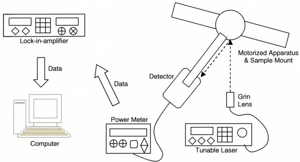
**Figure 2.4.3:** Variable incidence experimental setup.
