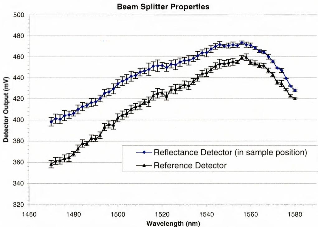
**Figure 2.3.5:** Plot portraying the beam splitting properties of the cube over the laser operating spectrum at  $100\mu\text{W}$  output power.
