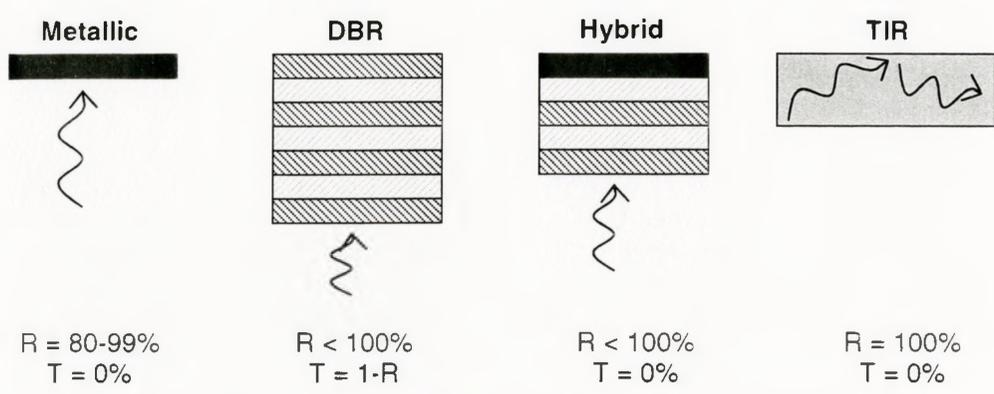
**Figure 1.1.3:** Schematic illustration of different types of reflectors.
