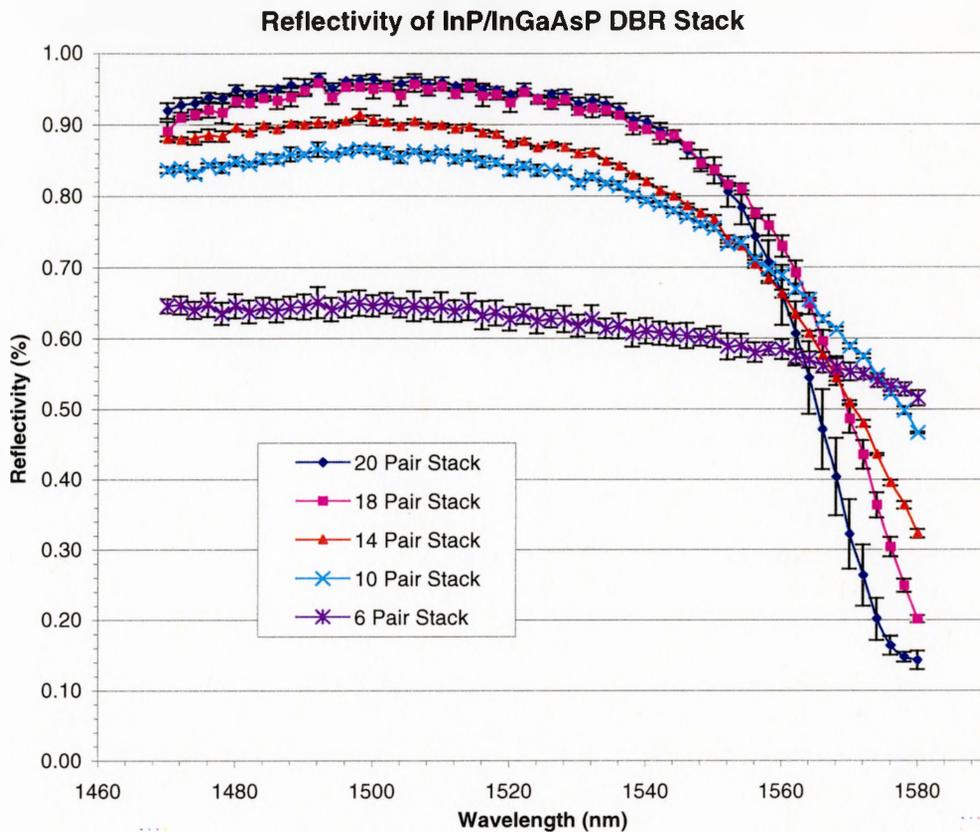
**Figure 4.2.4:** Normal incidence reflectivity measurement of InP/InGaAsP DBR stack with various numbers of pairs.
