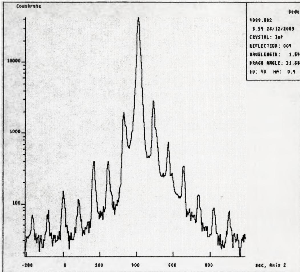
**Figure 4.6.1:** X-ray scan of a 20 pair InP/InGaAsP DBR stack.
