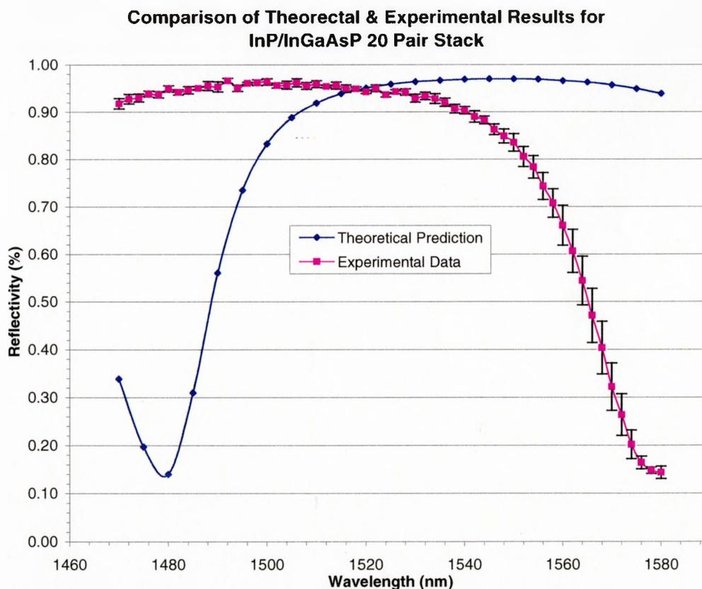
**Figure 4.2.2:** Comparison of original theoretical values used to calculate reflectivity for 20 pair stack with experimentally gathered curve.
