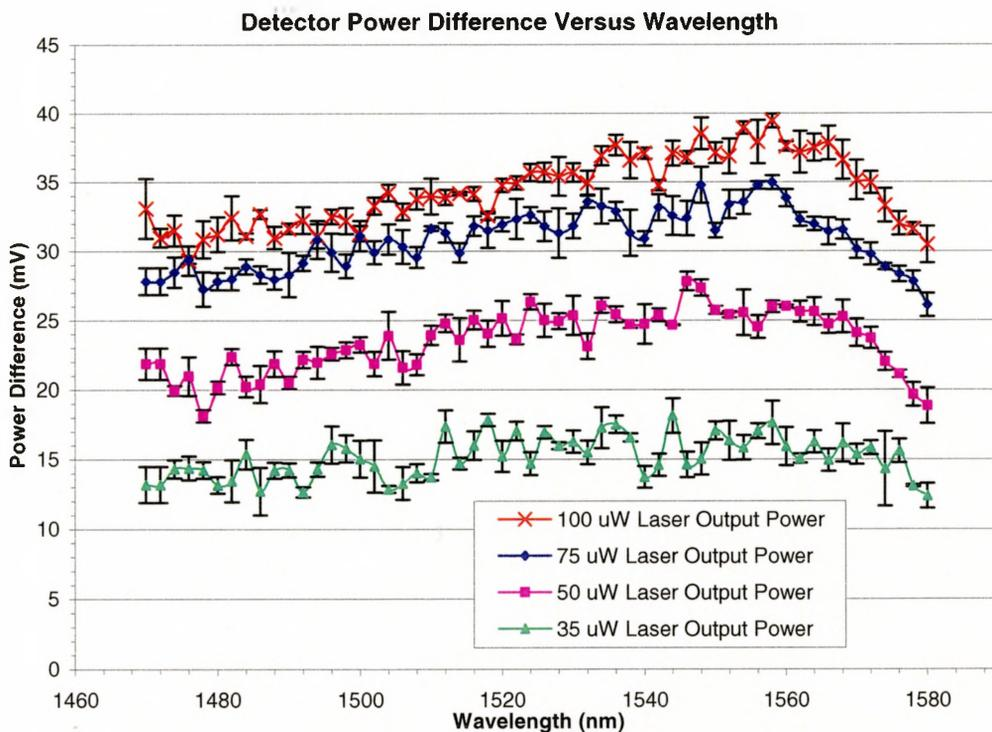
**Figure 2.3.4:** Varied laser output power and the resultant power difference between detector outputs.
