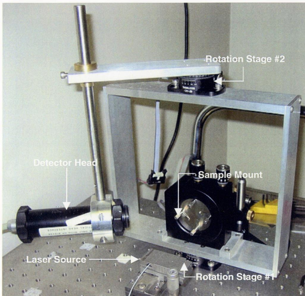
**Figure 2.4.2:** Rotation stage apparatus.
