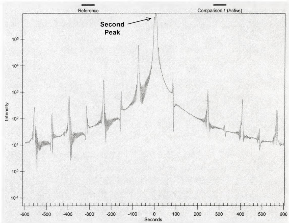
**Figure 5.4.5:** X-ray simulation of the 20 pair GaAs/InGaP DBR stack with a slight thickness change using Bede Version 3.0 software.
