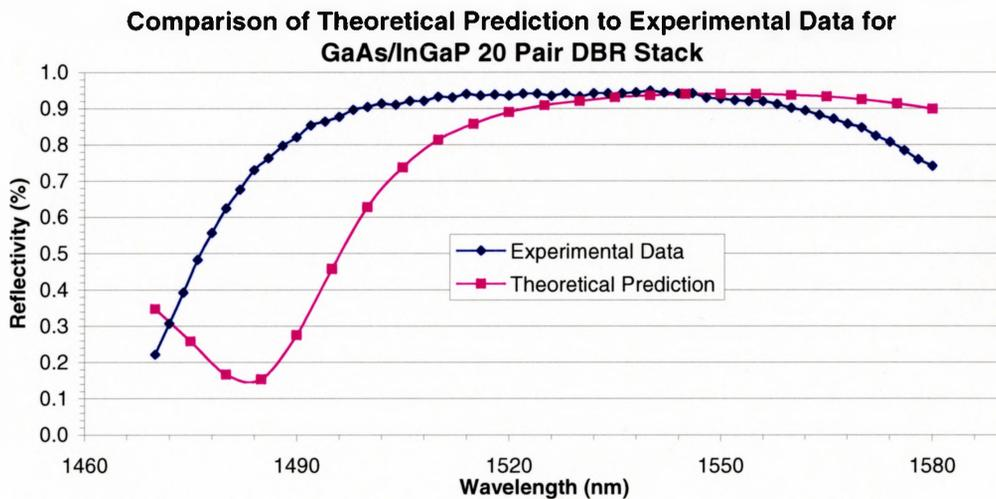
**Figure 5.2.3:** Theoretical predictions of 20 pair GaAs/InGaP DBR stack with experimentally obtained data.
