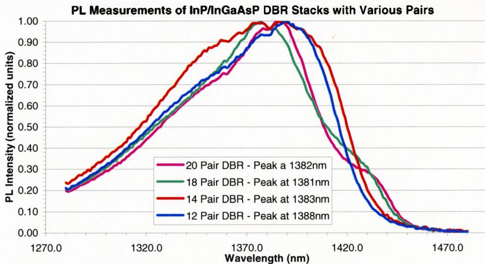
**Figure 4.7.2:** PL measurements taken from DBR stacks.
