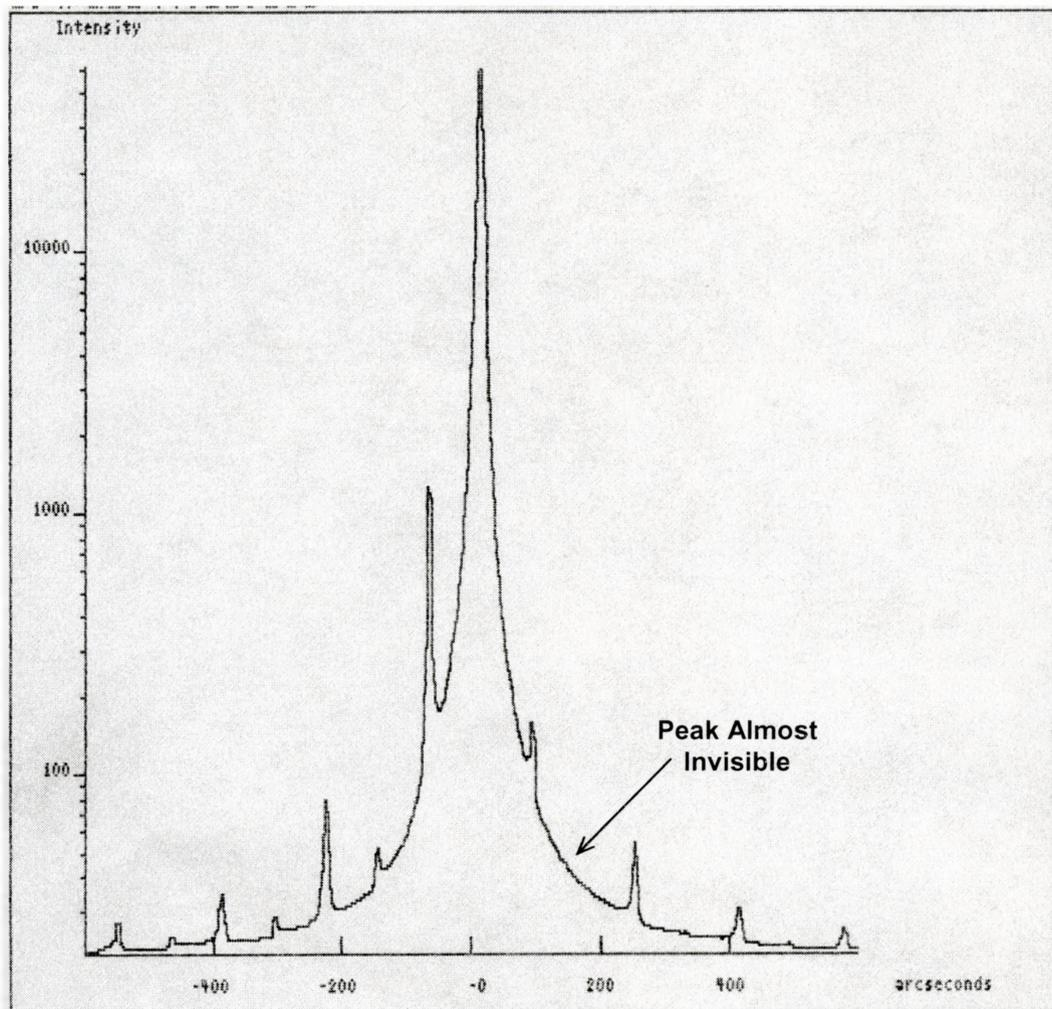
**Figure 5.4.2:** X-ray simulation of the 20 pair GaAs/InGaP DBR stack using Bede original software.
