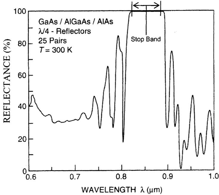
**Figure 3.1.3:** Reflectance of an AlGaAs/AIAs DBR with 25 pairs [3].
