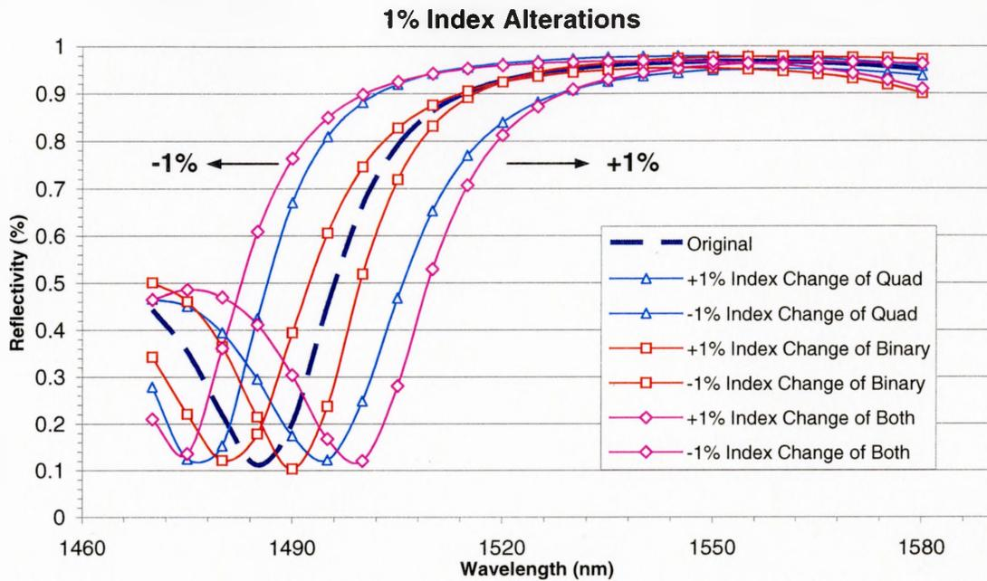
**Figure 4.3.1(b):** Observed effects of a  $\pm 1\%$  alteration of index of refraction for 20 pair DBR stack.
