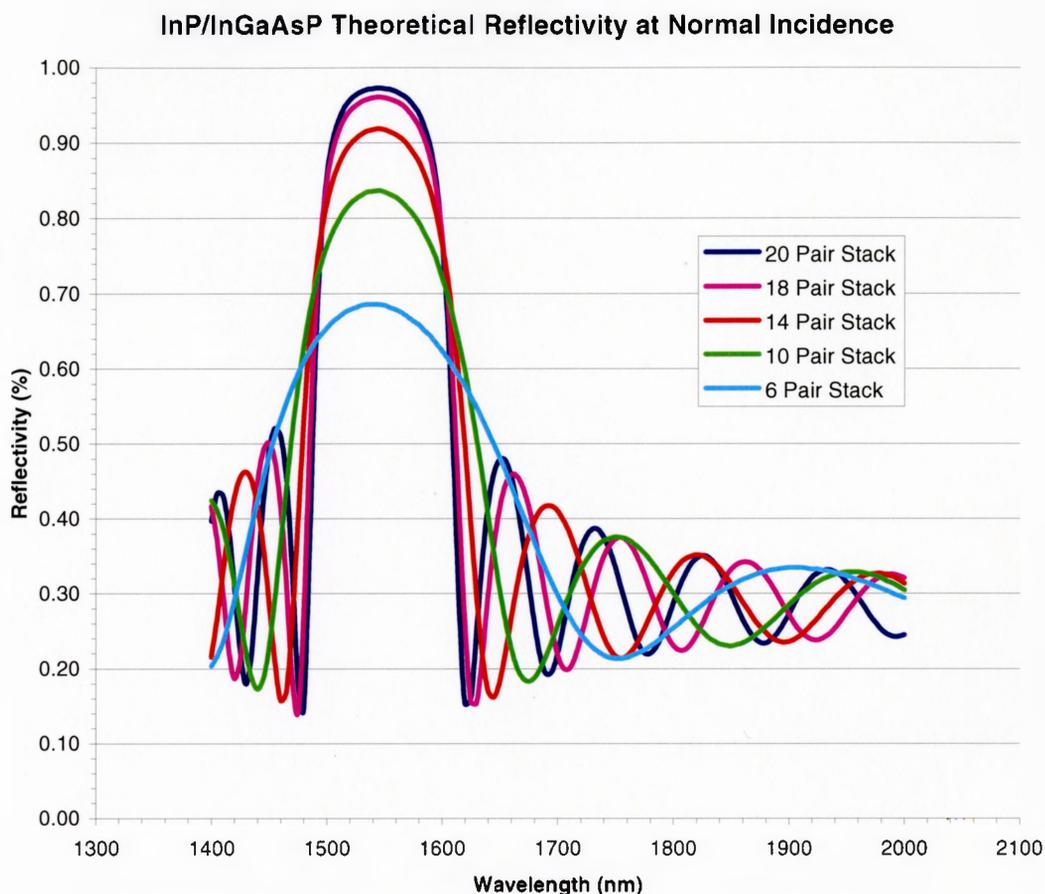
**Figure 4.2.3:** Theoretical Reflectivity of InP/InGaAsP DBR stack with various numbers of pairs at normal incidence.
