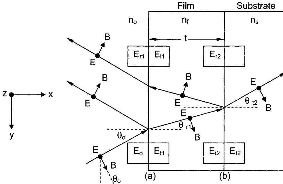
Figure 3.4.1: Reflection of a beam from a single layer film [13].
