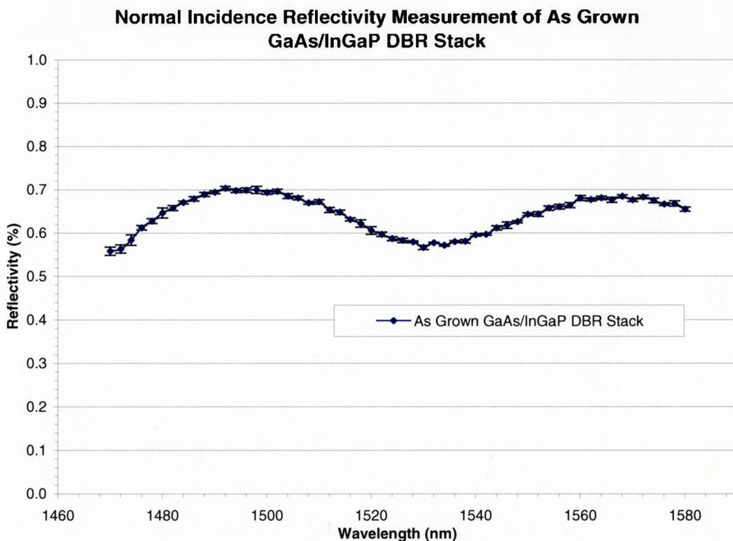
**Figure 5.2.1:** Normal incidence reflectivity measurements of as grown DBR stack with 20.5 pairs.
