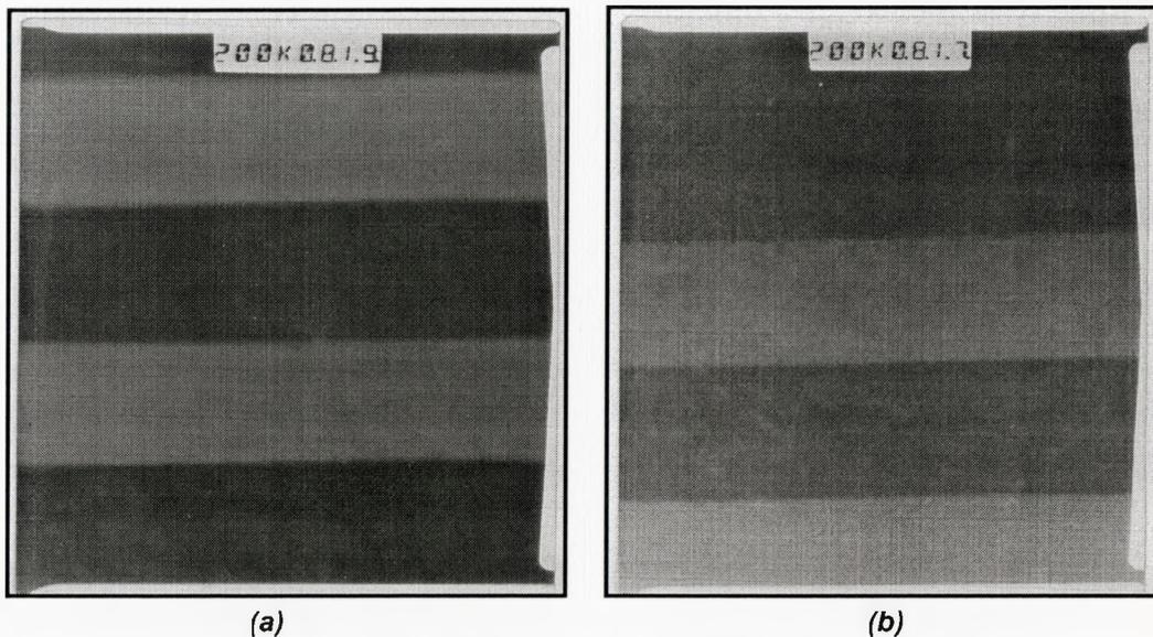
**Figure 4.5.3:** TEM micrographs of (a) bottom three layers and (b) top three layers of InP/InGaAsP DBR stack.
