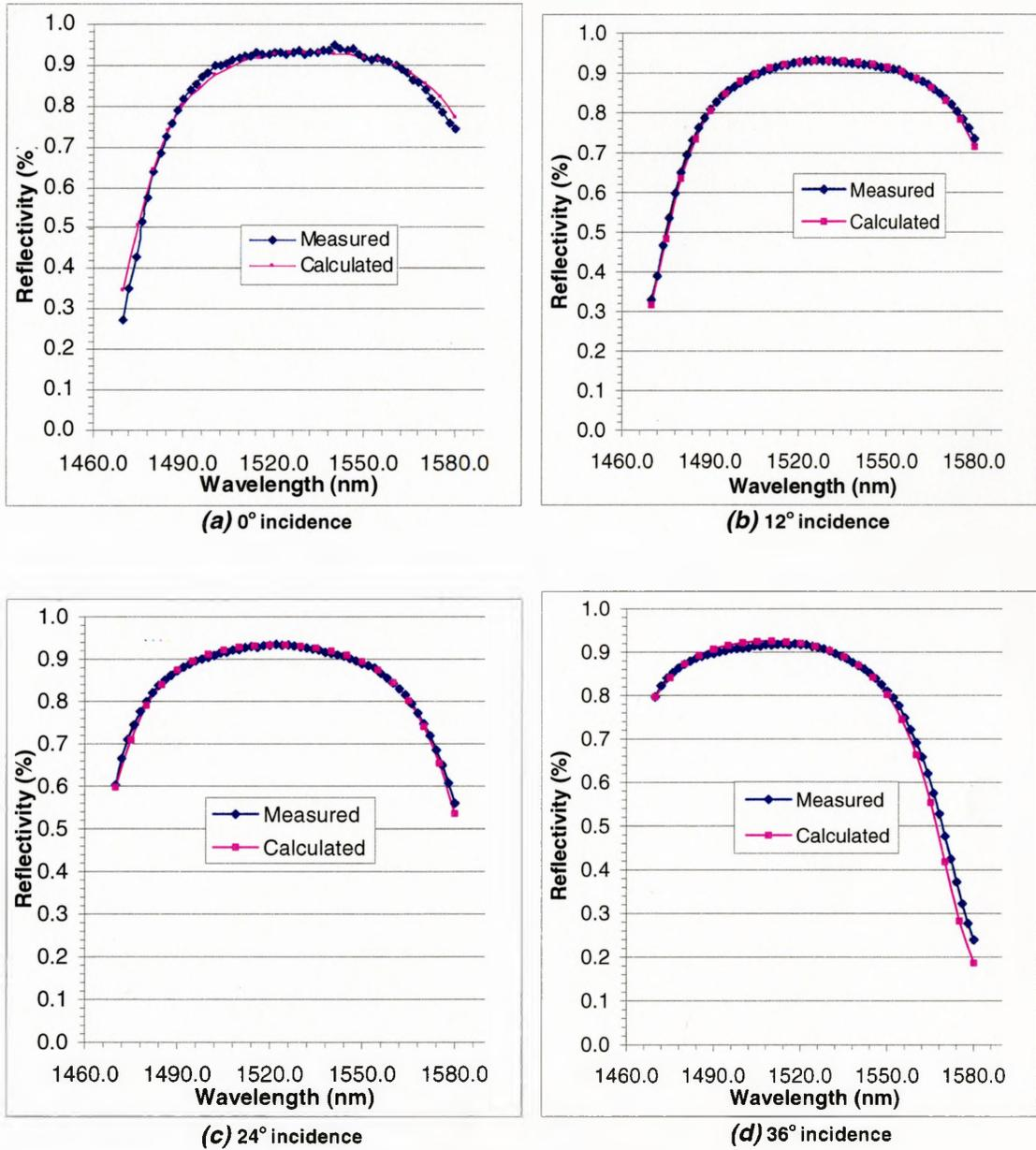
**Figure 5.3.2:** Theoretical fit to experimental data of 19 pair GaAs/InGaP DBR stack.
