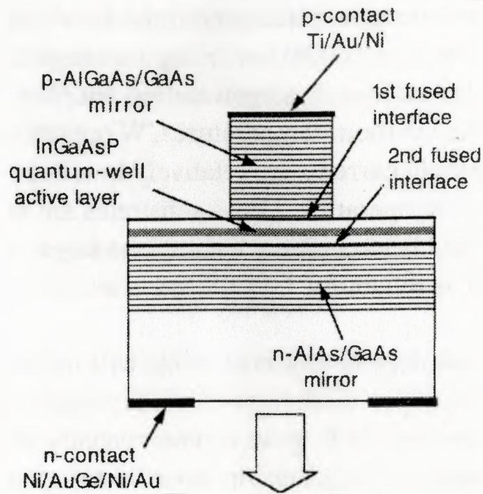
**Figure 3.1.1:** Cross-section diagram of a 1.55 $\mu\text{m}$  wavelength VCSEL with fused AlGaAs/GaAs mirrors [12].
