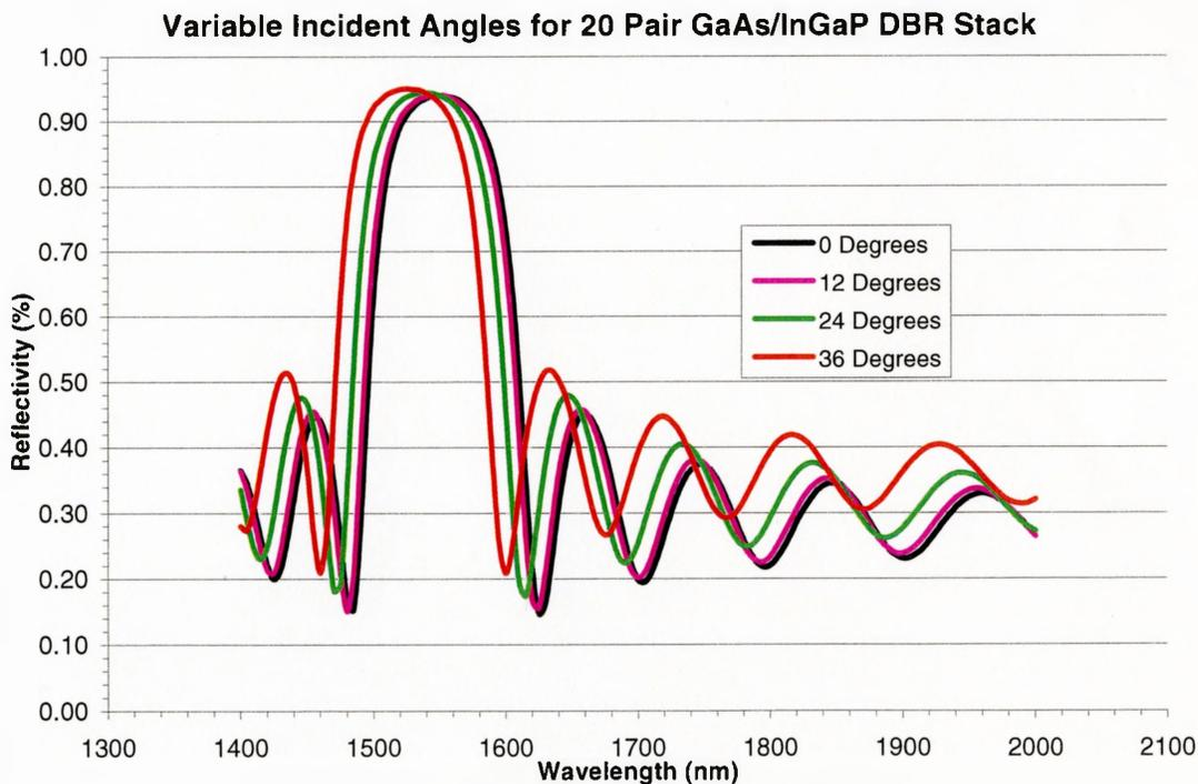
**Figure 5.2.5:** Variable incident reflectivity measurement of 20 pair GaAs/InGaP DBR stack.
