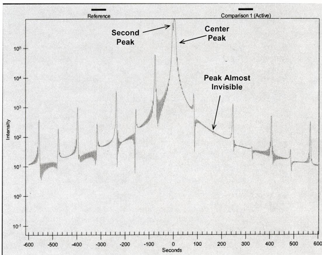
**Figure 5.4.3:** X-ray simulation of the 20 pair GaAs/InGaP DBR stack using Bede software Version 3.0.
