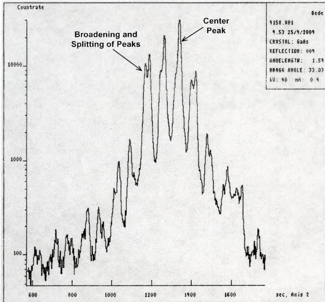
**Figure 5.4.1:** X-ray scan of the 20 pair GaAs/InGaP DBR stack.
