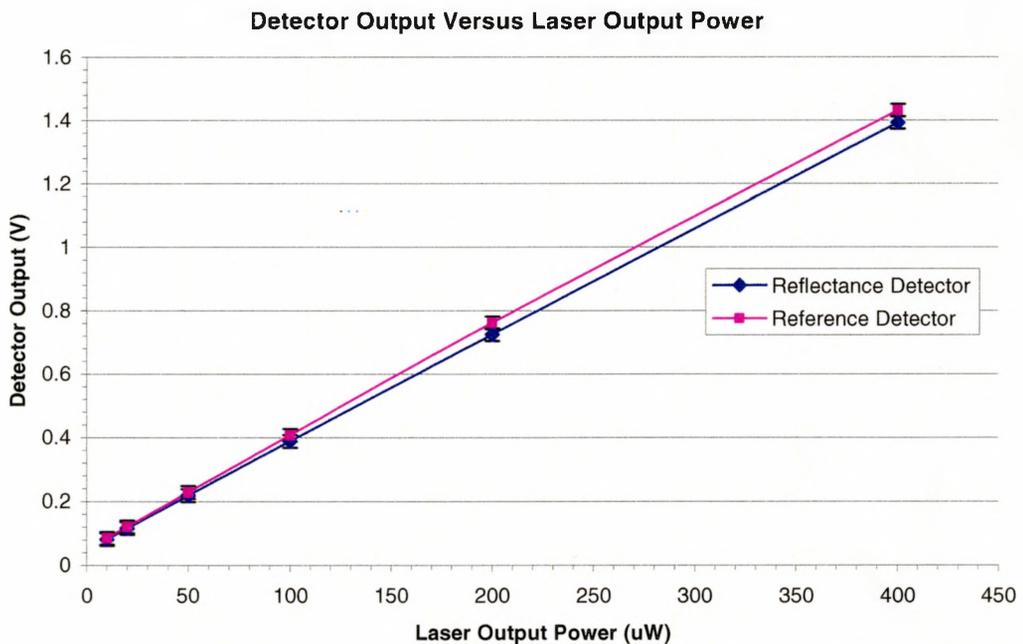
**Figure 2.3.2:** Plot displaying linear power response of both detectors at 1550nm.
