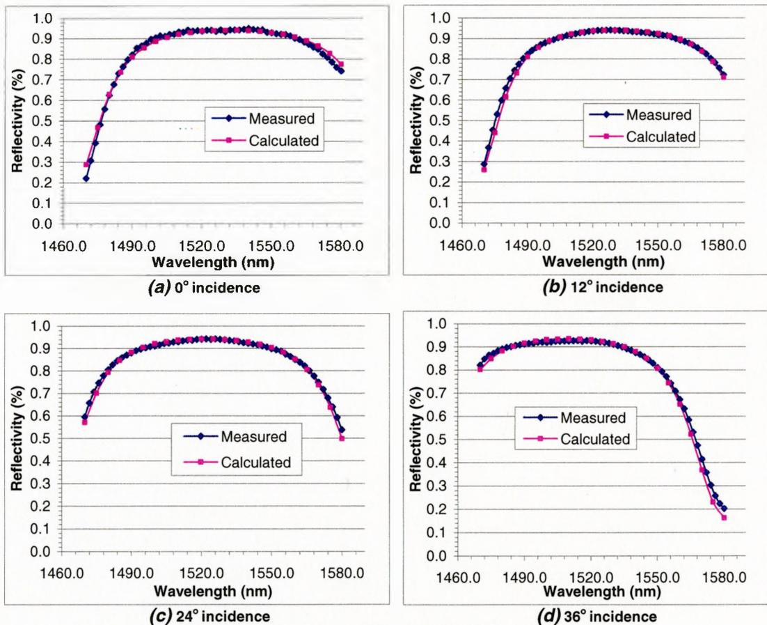
**Figure 5.3.1:** Theoretical fit to experimental data of 20 pair GaAs/InGaP DBR stack.
