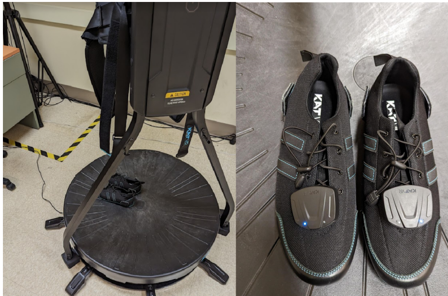
Figure 2.2: This figure shows the KAT Walk C Treadmill (Left) along with the accompanied KAT Walk Shoes (Right).
