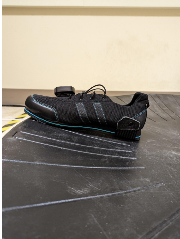
Figure 2.3: This figure depicts the incline of the KAT Walk C surface when the shoe is near the edge of the surface.
