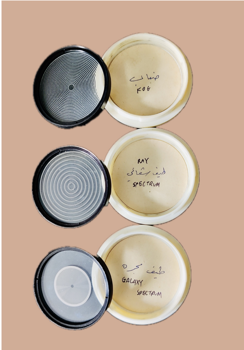
Fig. 2: The three lens filters of Zenit camera named in both Arabic and English which are Fog, Spectrum and Galaxy Spectrum.
