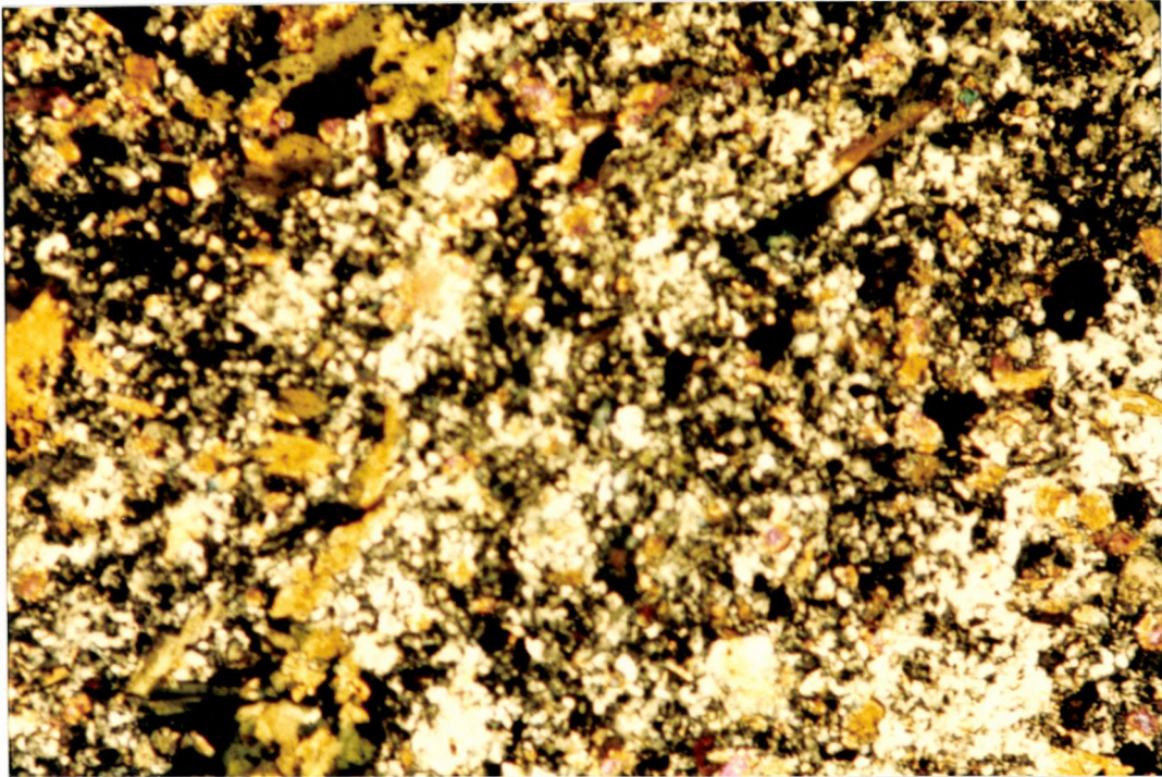
PLATE 5-2 The groundmass to the granodiorite clasts is dominated by hornblende and albite. Polarized light, x63. The field of view is 1.0 x 1.5 mm.
