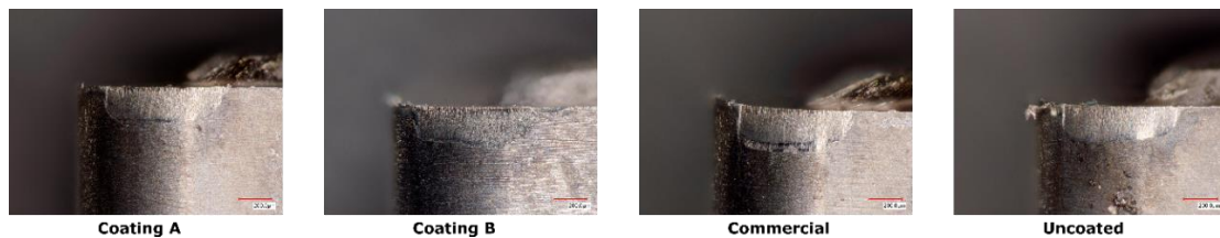
Figure 4.11 3D tool wear images of tools at a cutting length of approximately 600 m during the dry finish turning of AISI 304
