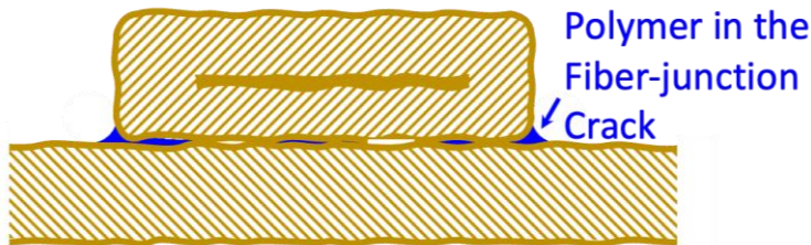
Figure 19 An illustration of a cross section of 90-degree crossed fibres showing the proposed polymer distribution after impregnation and curing. The crosslinked polymer in the fibre-junction crack may inhibit crack growth.
