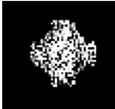
Figure 6.1.8: subchannel void fraction map using the images in Figure 6.1.4. Display range [0, 1]. The image displays non-realistic contrast since a value threshold is used.
