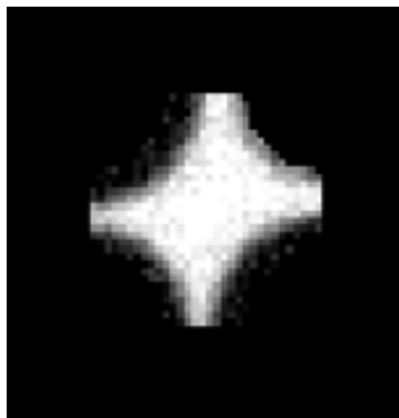
Figure 6.1.9: subchannel void fraction map for the McMaster simulation using the images in Figure 6.1.6Figure 6.1.4. Display range [0, 1].
