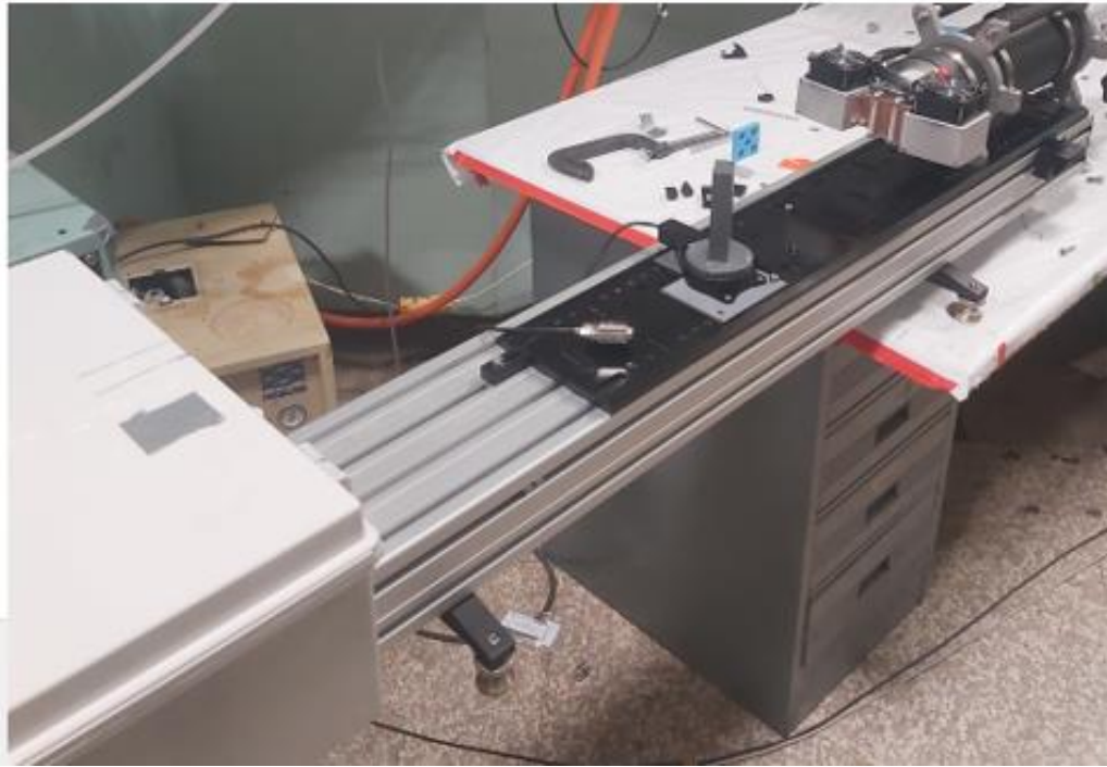
Figure 5.1.18: benchtop testing unit mounted to an aluminum alignment beam with detector box (white, left) rotation stage (middle) and neutron generator (right).
