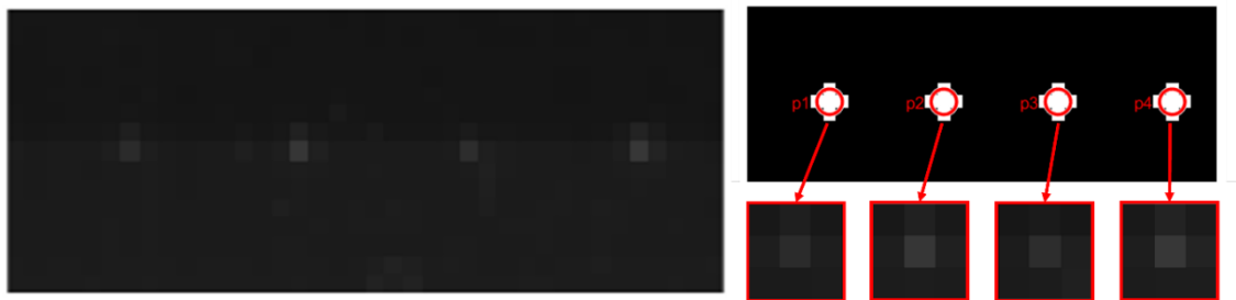
Figure 44: Automatic output port detection using a MATLAB script.
