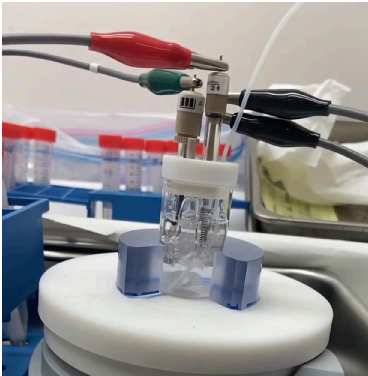
Figure A3 - Electrolytic Cell used to reduce Tc(VII) to Tc(IV). The RE is to the left with the green alligator clip. The Pt WE is in the middle with the two black alligator clips. The CE is in the front with the red alligator clip.
