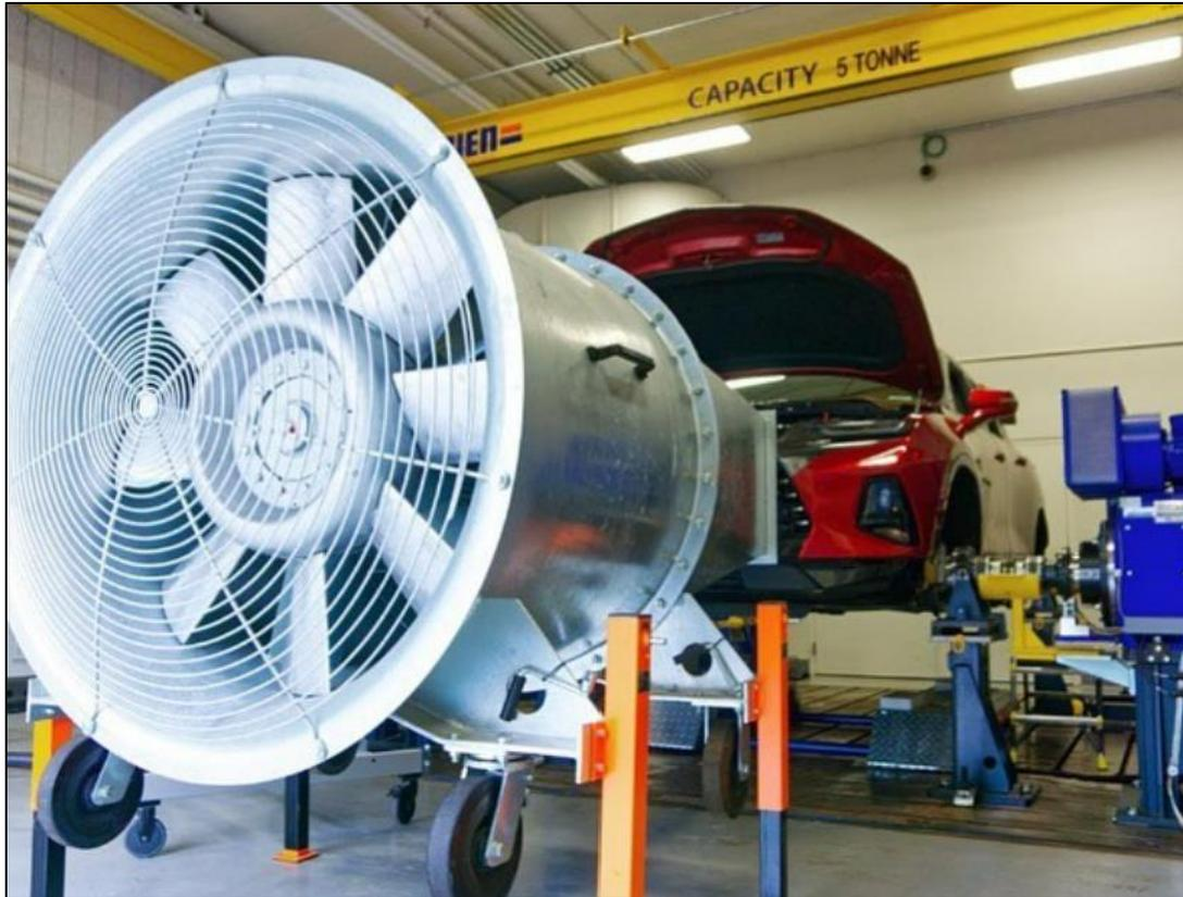
Figure 27: MAC Team Vehicle on Chassis Dynamometer
