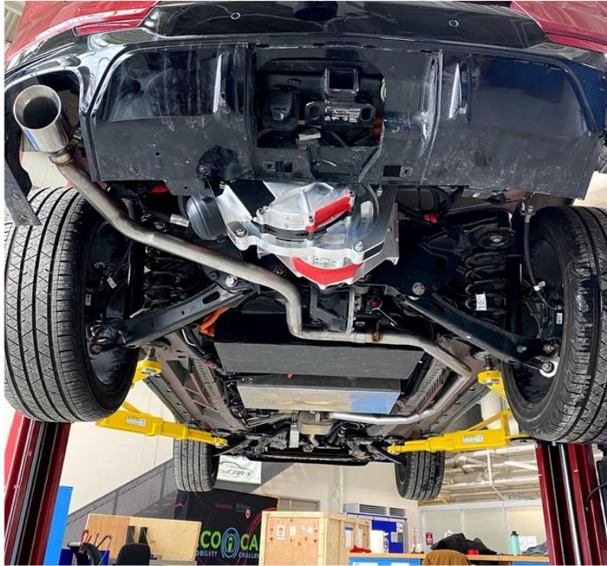
Figure 7: MAC Team Vehicle Fully Integrated P4 Architecture
