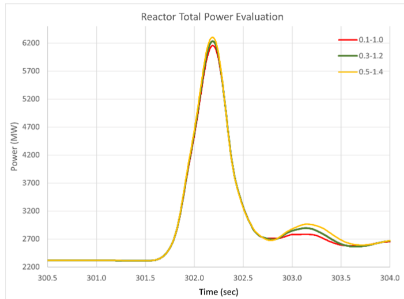
Figure 6.12: Reactor total power production with different BPV actuation times
