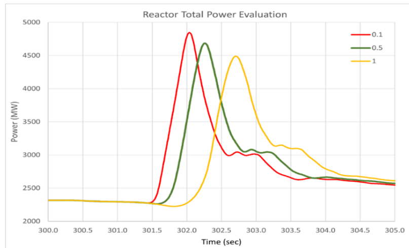
Figure 6.5: Effect of different TSV closing speeds on reactor power response
