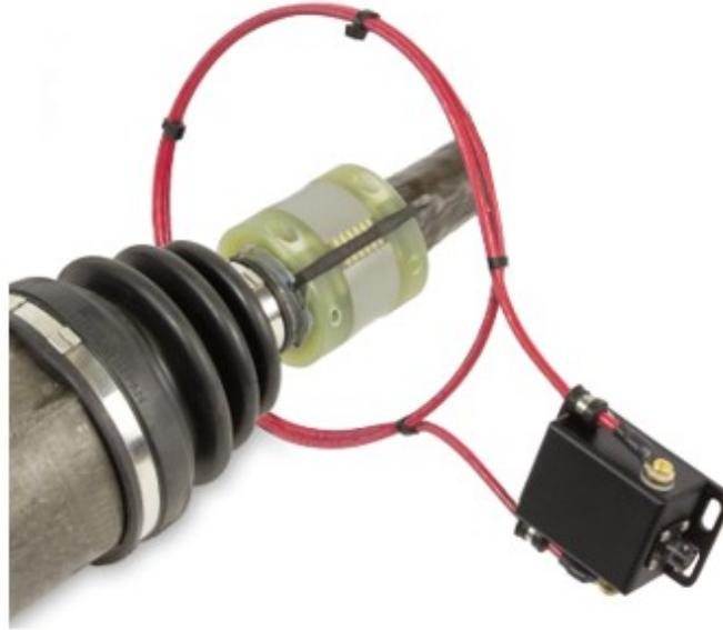
Figure 11.2: Induction based telemetric setup [11]
