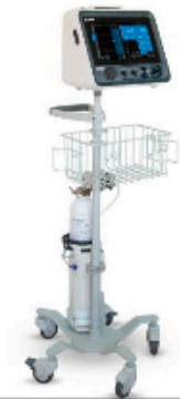
Figure 1. The metabolic cart QNRG is used to measure the indirect calorimetry.
