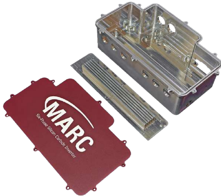
Figure 7.1: Manufactured inverter housing and heat sink.
