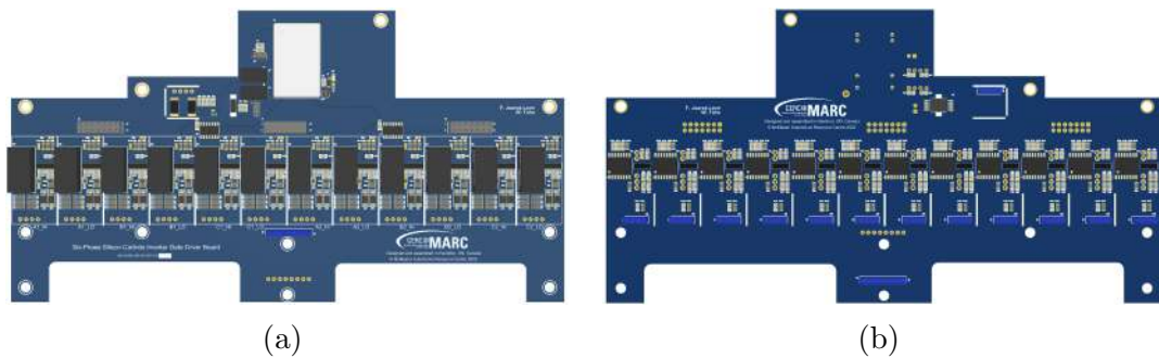
Figure 6.18: Gate driver board 3D view. (a) Top view. (b) Bottom view.
