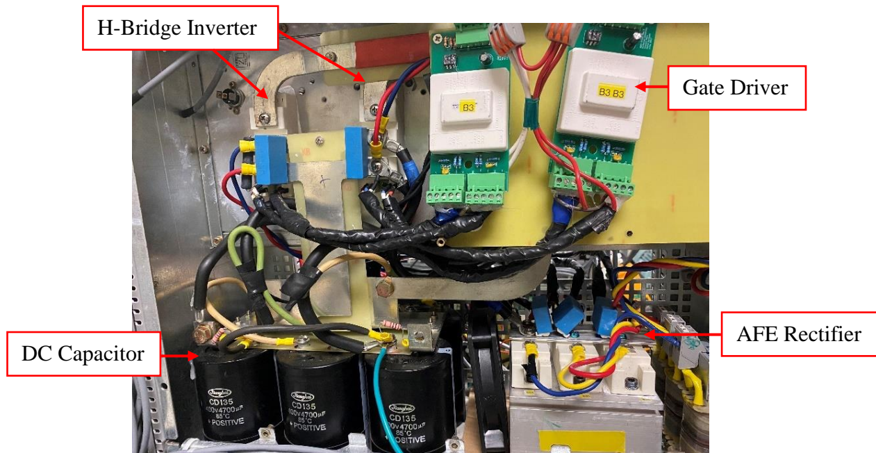
Fig.7.3. The Structure of Power Cell
