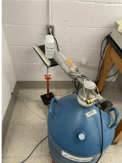
*Figure 11: The measurement of Na-24 volume source. In this figure, the bottle is placed 15 cm from the detector, and the center of the detector is lined up with the midline of the liquid.*
