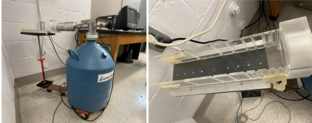
*Figure 3: The Ortec N-type HPGe detector used for in-lab measurement. The detector part is attached to the blue LN2 dewar, shown on the left. The source holding rack is shown on the right.*
