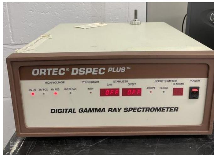
*Figure 4: The Ortec DSPEC Plus gamma spectrometry system.*
