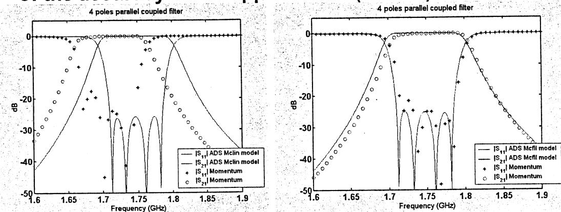
**Coarse model 1:** cascade of coupled line sections without any discontinuity effects.
