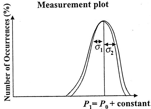
Constant = deviation of measurements in jig compared to the simulation (demoboard)
