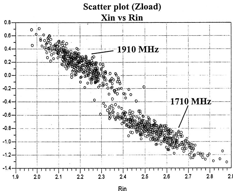
The input impedance of the matching network is the load impedance which is seen by the power amplifier.
