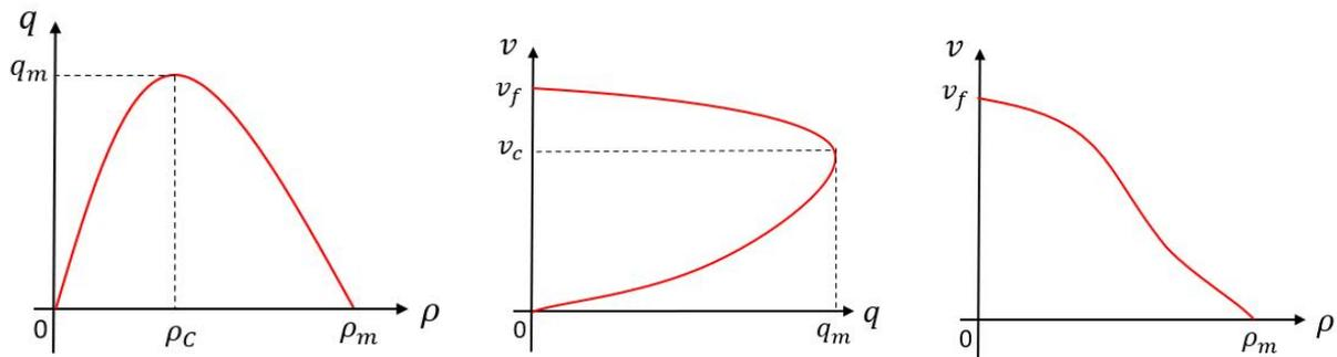
**Fig 4.2.1: The Van Aerde Traffic Stream Model**
