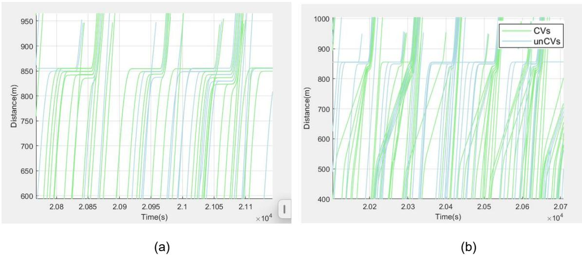
**Fig. 4.3.1: Individual vehicle dynamics at the first intersection: (a) trajectories with the pre-time signal, (b) trajectories with the CVSC system**
