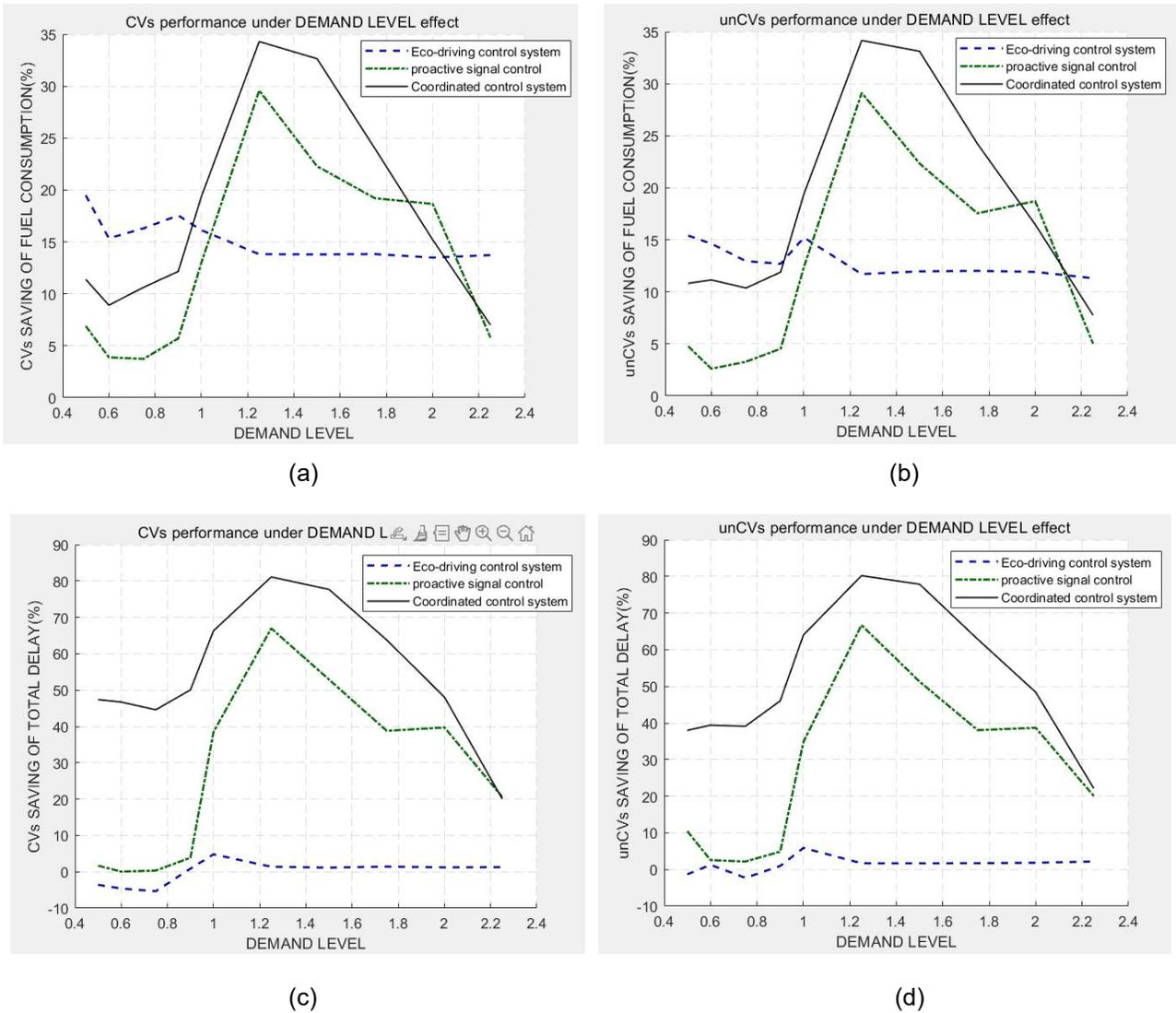
**Fig. 4.3.2.1: Benefit comparison at different demand levels: (a) savings in fuel consumption for CVs, (b) savings in fuel consumption for non-CVs, (c) savings in travel time delay for CVs, and (d) savings in travel time delay for non-CVs**
