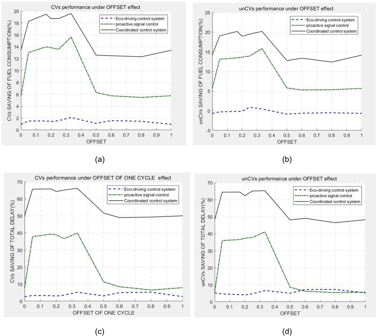
**Fig. 4.3.4.1: Benefit comparison at different offsets: (a) savings in fuel consumption for CVs, (b) savings in fuel consumption for non-CVs, (c) savings in travel time delay for CVs, and (d) savings in travel time delay for non-CVs**
