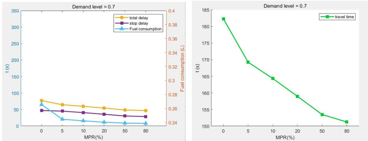
Fig. 4.3.5.3, Average delay and travel time as a function of MPR for saturation of 0.7
