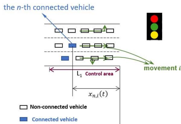
**Fig. 3.3.1: Proactive control at one signalized intersection**
