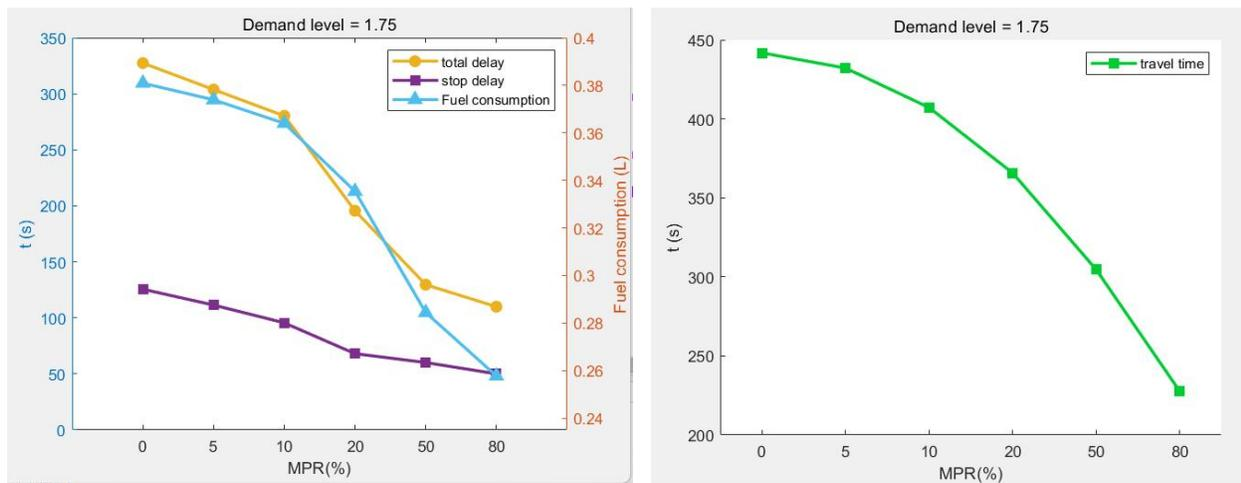
Fig. 4.3.5.2, Average delay and travel time as a function of MPR for saturation of 1.75
