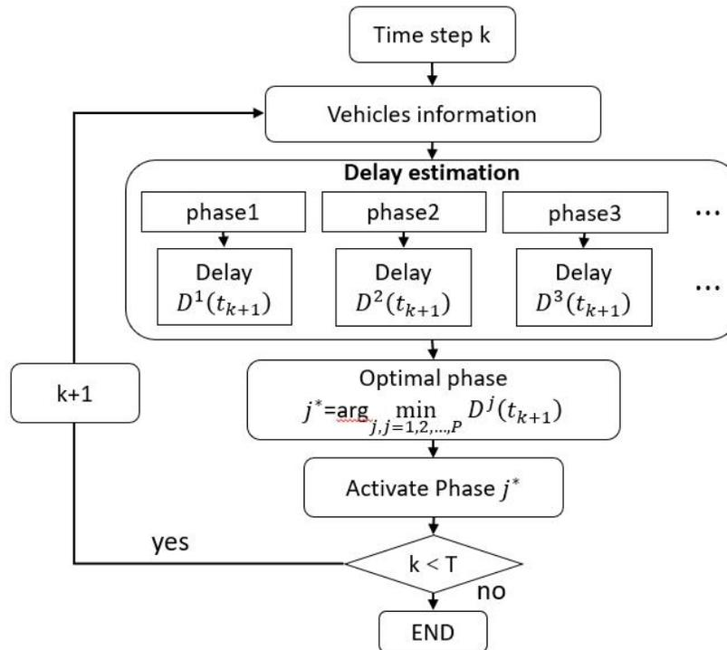
**Fig. 3.3.2: Flow chart of the proactive signal control system**
