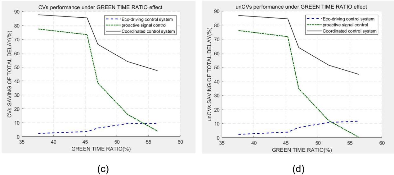
**Fig. 4.3.3.1: Benefit comparison at different green timing ratios: (a) savings in fuel consumption for CVs, (b) savings in fuel consumption for non-CVs, (c) savings in travel time delay for CVs, and (d) savings in travel time delay for non-CVs**
