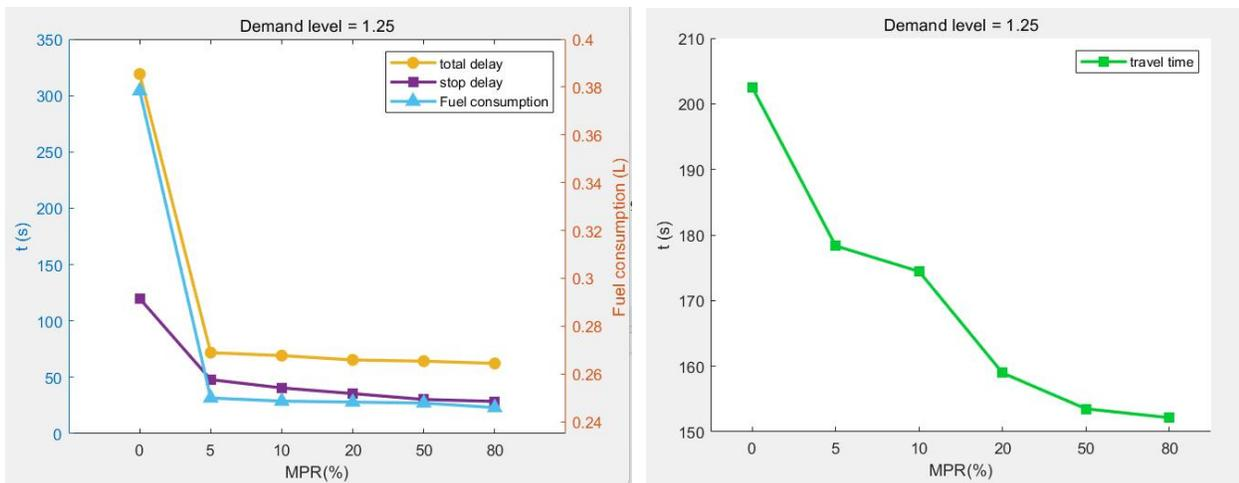
**Fig. 4.3.5.1, Average delay and travel time as a function of MPR for saturation of 1.25**
