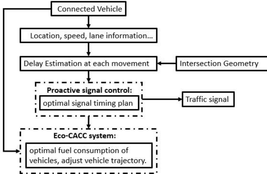
**Fig. 3.4.2 The framework of the CVSC system**
