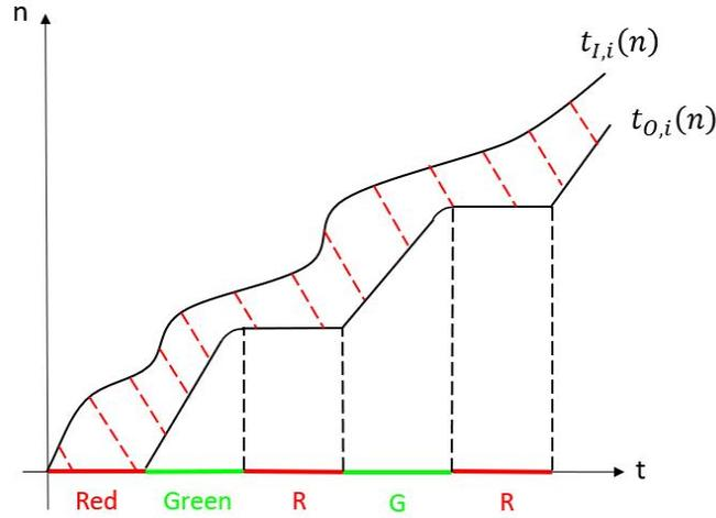
**Fig. 3.2.2: Cumulative flow rates and delays**
