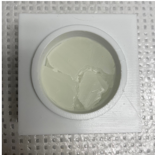
Figure 3.5: Sample holder used for ex vivo sample measurement. Notice the wax fitted within the phantom, which was added to ensure a similar scattering environment to water.
