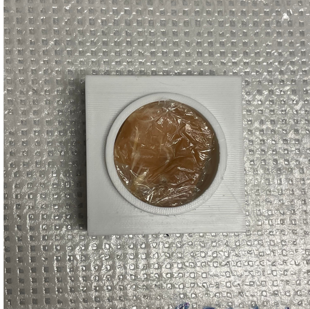
Figure 3.6: Sample holder with mounted rat skin sample over wax layer.
