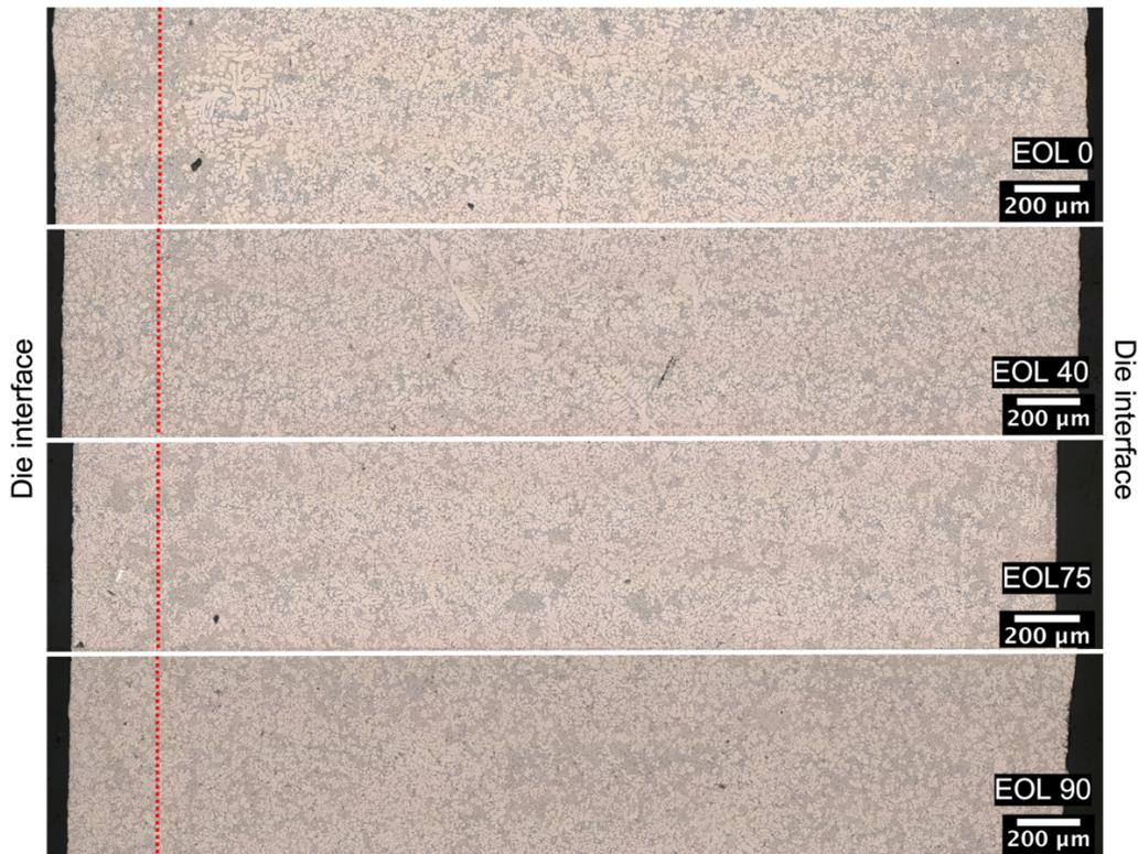
Figure 5.1: Microstructure images of each EOL alloy obtained by LOM, cross section view. Red dotted lines demark the interface between the skin (located on either side) and the core
