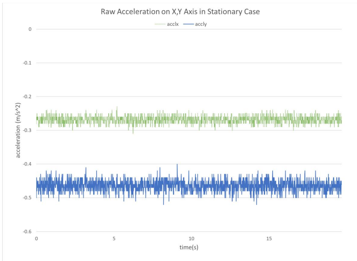
Figure 8 The raw accelerometer data from IMU in the stationary case
