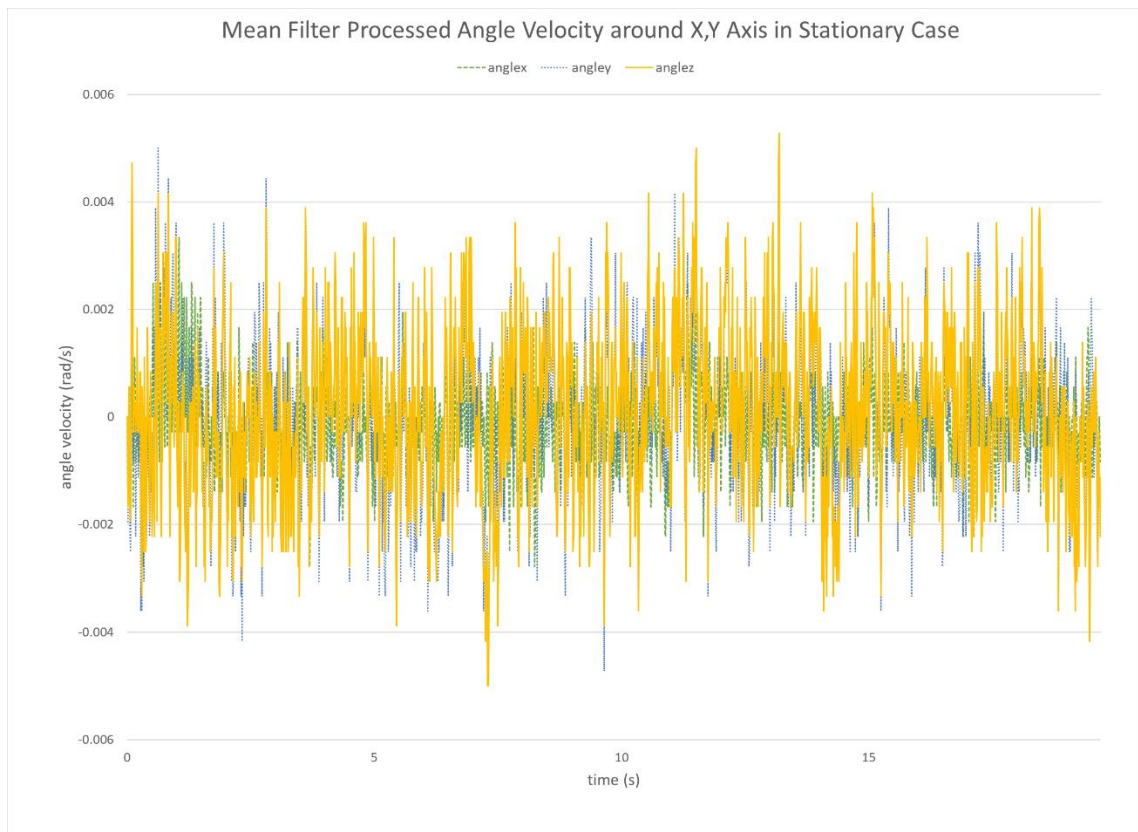
Figure 15 Mean filter processed angle velocity around x,y axis in stationary case
