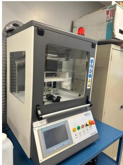
**Figure S3.6** Photograph of NE300 electrospinner.
