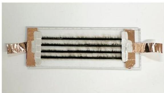
**Figure S5.6** The parallel line design for the PC-LIG temperature sensor with copper tape connected by silver paste
