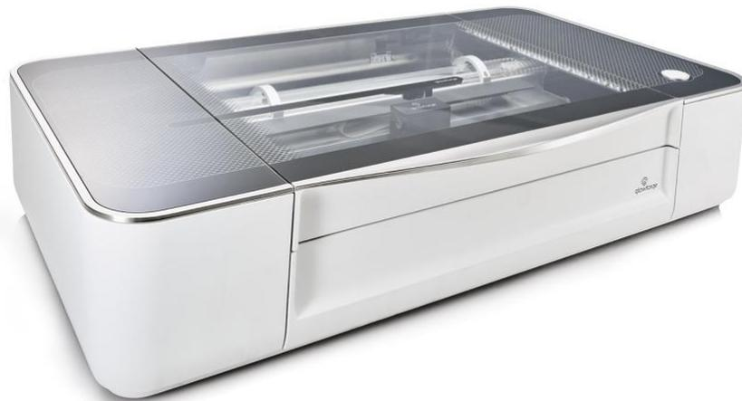
**Figure S5.8** Photograph of Glowforge CO<sub>2</sub> laser machine.
