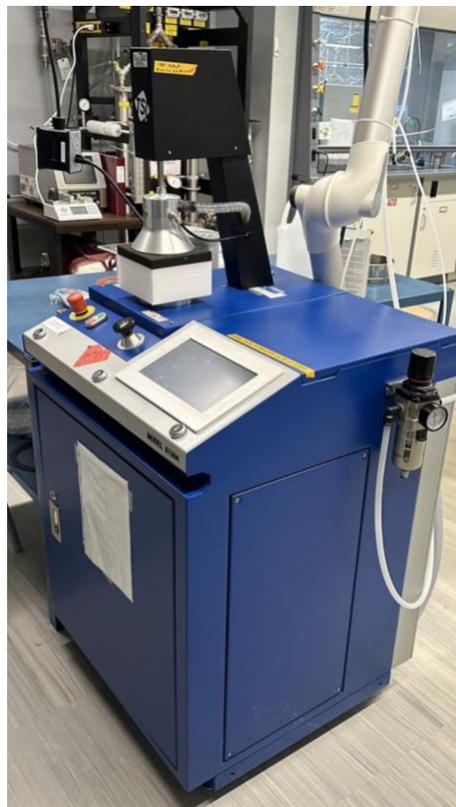
**Figure S3.7** Photograph of TSI 8130A for filtration.
