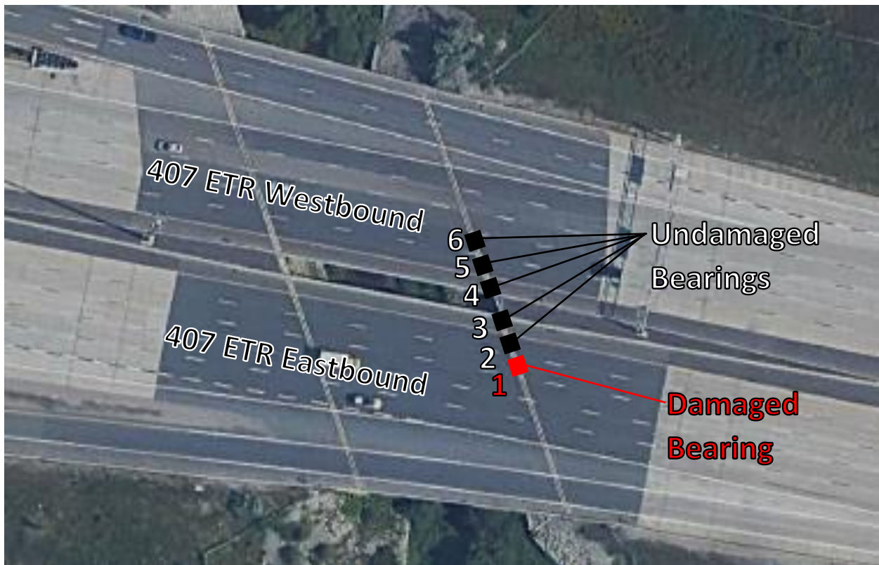
Figure 15: Location of bearings at German Mills Creek site; maps data: Google, Image Landsat/Copernicus
