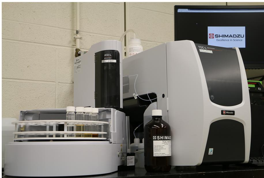
**Figure 2.10:** The Shimadzu TOC-LCPH instrument with autosampler used in this work.
