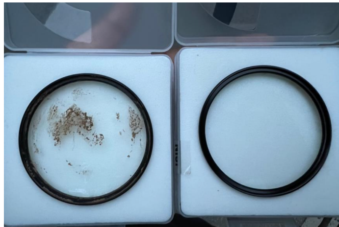
Figure 4.1: Glass filter adhered by dirt(left). Clean glass filter (right).
