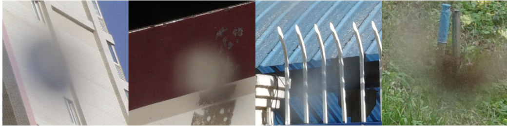
Figure 4.3: From left to right: raindrop sample, muddy raindrop sample, dirt sample, and tiny particle sample
