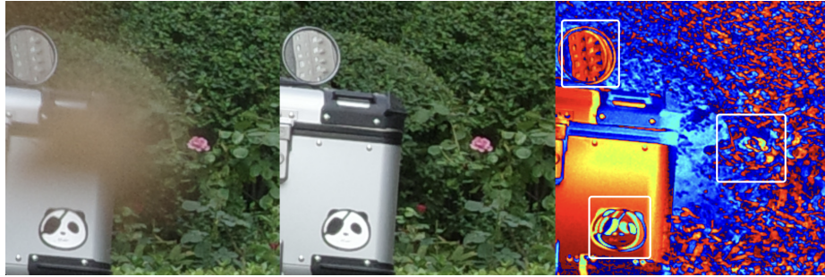
Figure 4.4: A comprehensive illustration of the image selection process. (white boxes denote pixel misalignments introduced by wind-induced disturbances). From left to right: Degraded image, ground truth, binary subtraction mask with apply with a heated map
