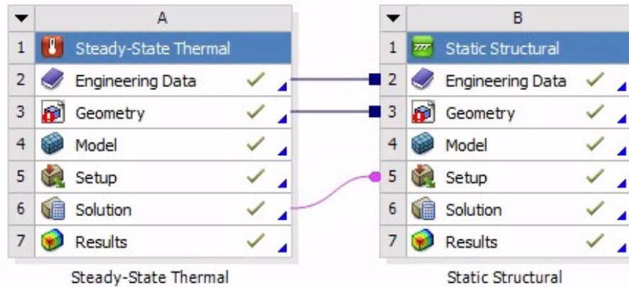
Figure 3.8: Coupled steady-state thermal and static structural units in ANSYS Mechanical packaging.
