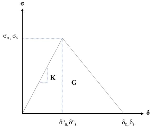
**Figure 4-3 Bilinear traction–separation law [39]**
