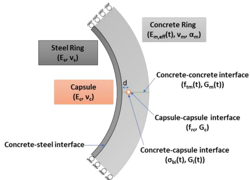
**Figure 4-2 Idealized model of the restrained shrinkage ring**
