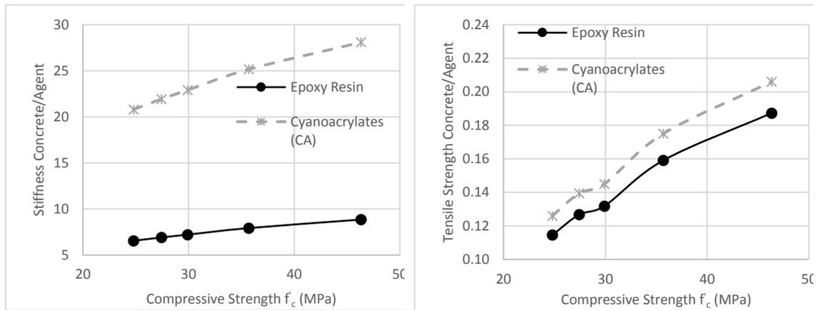
**Figure B-1 Mechanical properties of concrete with age and polymeric healing agents**
