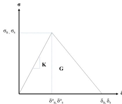
**Figure 2-3 Bilinear traction-separation law [93]**
