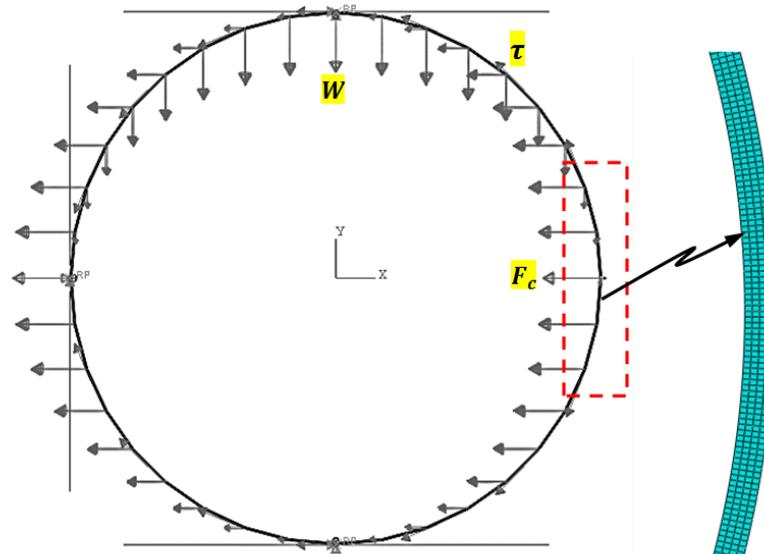
**Figure 3-2 FE model includes geometry, boundary & loading conditions, and mesh.**
