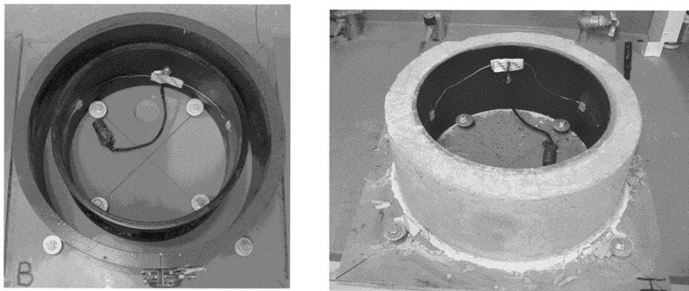
**Figure 4-1 Restrained shrinkage ring test, extracted from [18]**
