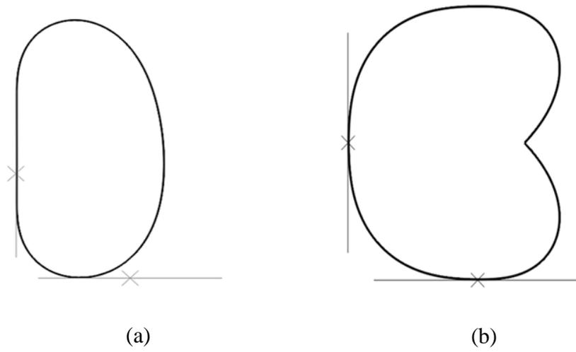
**Figure 3-3 Capsule failure modes deduced from the FE analysis, (a) Stretching and/or rupturing, (b) Punching**
