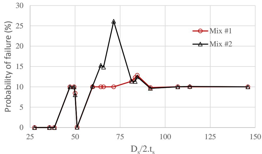
**Figure 3-4 Capsule radius-to-thickness probability of failure**
