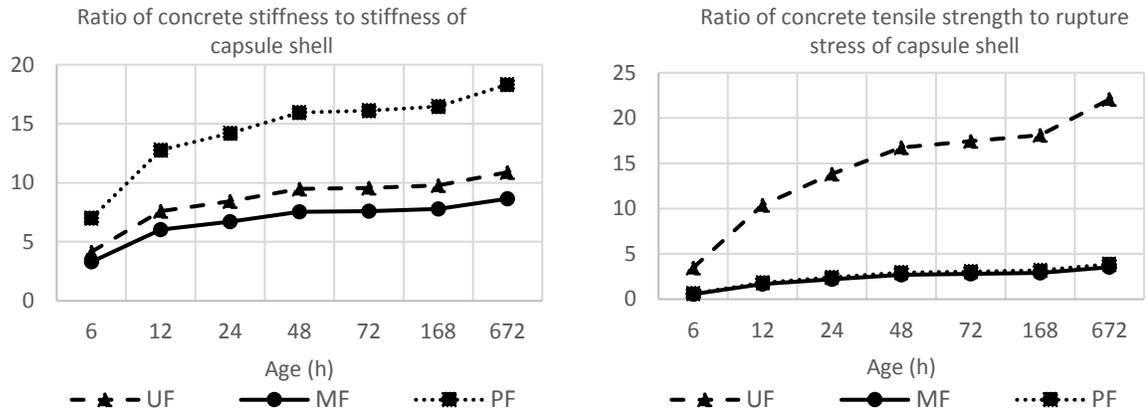
**Figure A-1 Mechanical properties of concrete with age and polymeric capsules**
