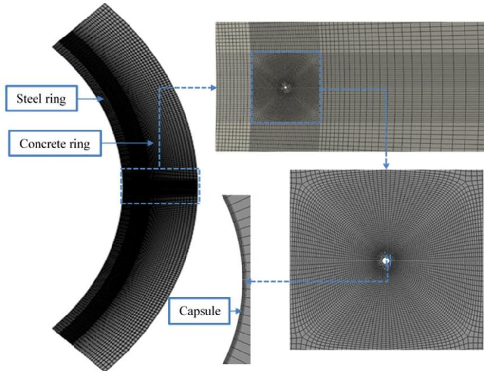
**Figure 4-4 FE mesh of the idealized restrained shrinkage ring with self-healing capsule**
