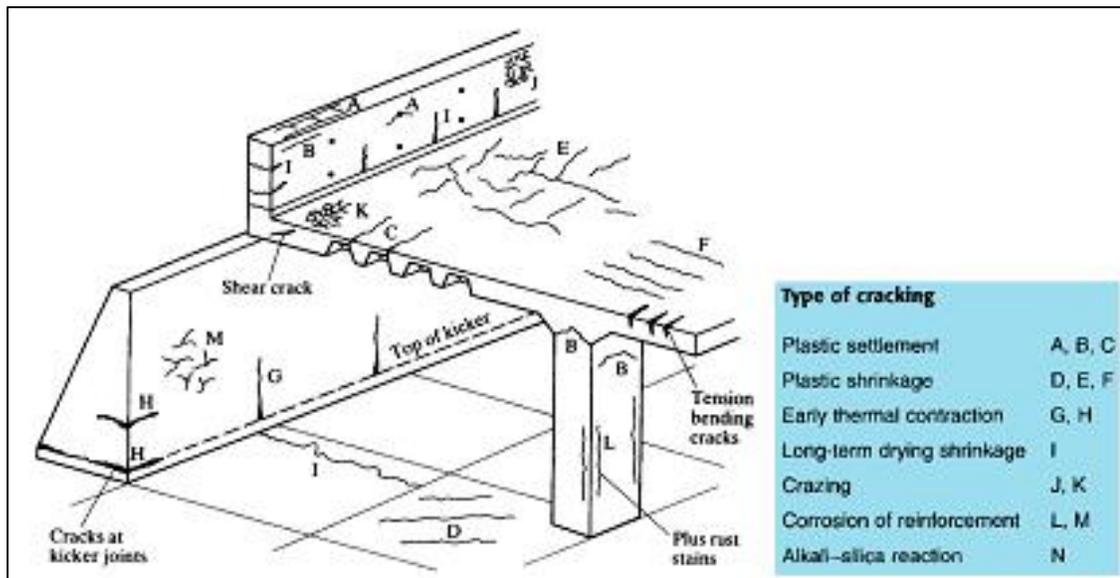
**Figure 1-1 Schematic representation of the various types of cracks in concrete [5]**
