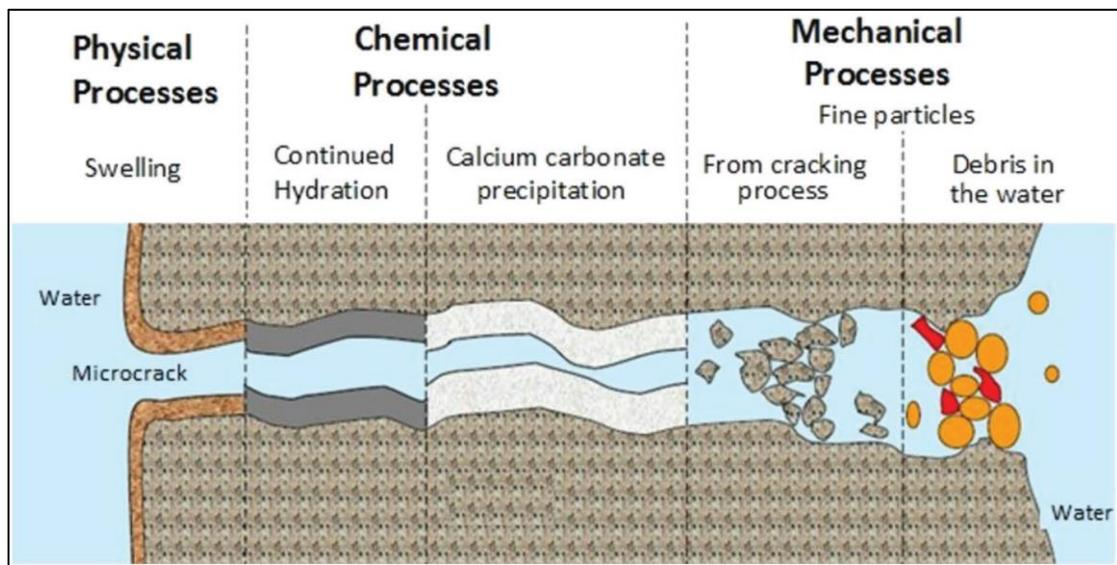
**Figure 1-2 Mechanisms of autogenous healing [25]**
