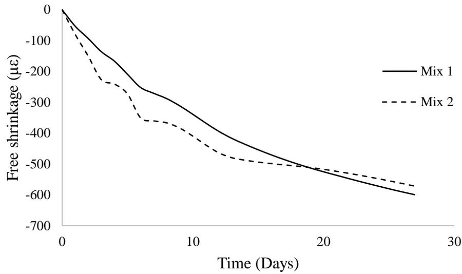
**Figure 4-5 Free shrinkage versus time for Mix 1 and Mix 2 [26]**
