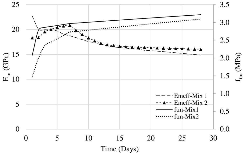
**Figure 4-7 Development of mechanical properties of concrete, reproduced from [26]**
