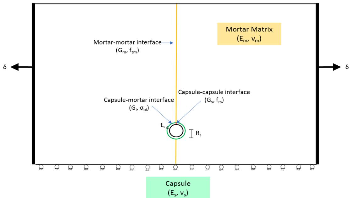
**Figure 2-1 FE model schematic view including geometry, boundary conditions, and loading conditions**
