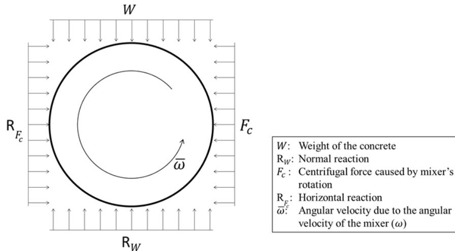
**Figure 3-1 Schematic model of a single capsule in a concrete mixer**
