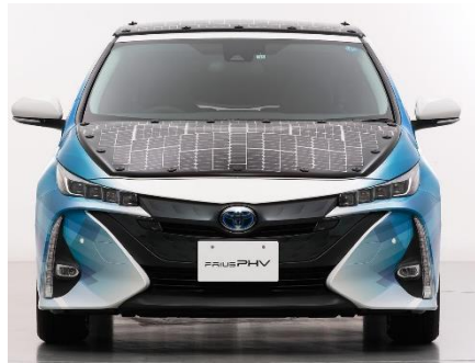
Figure 1-1: Prototype EV with on-board solar generation [8]
