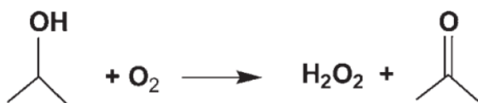
Figure 1-8: Oxidation of a secondary alcohol for the Synthesis of \text{H}_2\text{O}_2 , with permission from [2], Copyright 2006, Wiley and Sons.
