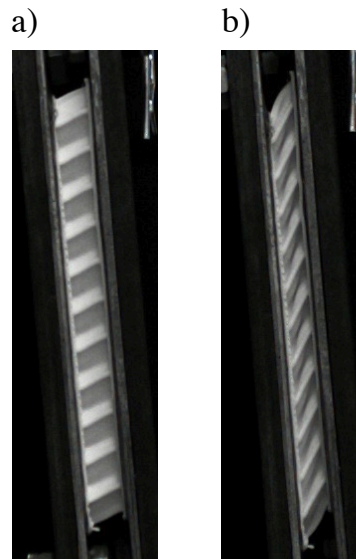
Figure 2.18: Deformation Patterns of Honeycomb Under Shear Loading
