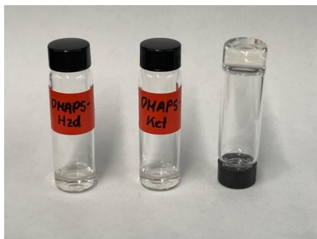
Figure S5.5: Photographs of hydrazide (DMAPS-Hzd) and ketone (DMAPS-Ket) precursor polymers and the resulting hydrazone-crosslinked DMAPS hydrogel (10 wt% precursor polymer, after 2 minutes).
