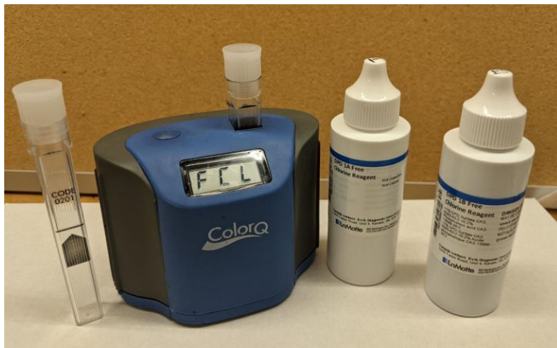
Figure 4-3: ColorQ PRO 7 Hand-Held Photometer commercial DPD-based colorimetric test kit with accompanying test tubes and chlorine reagents.
