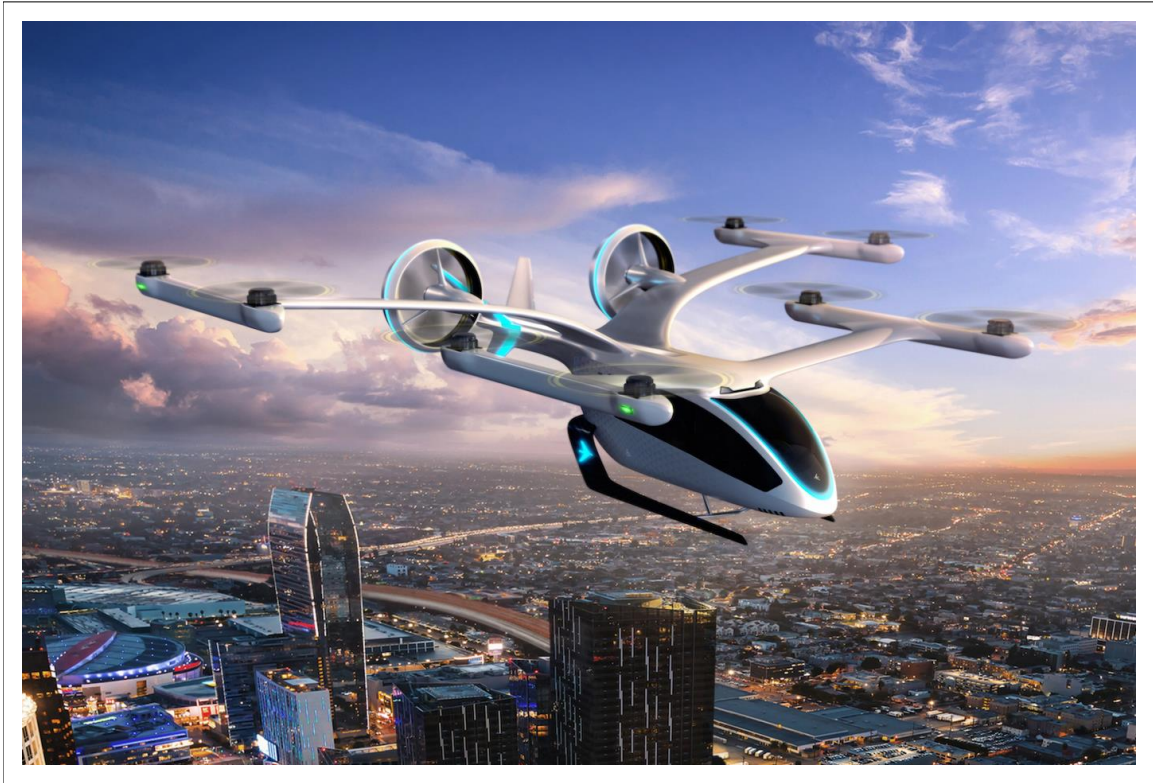
Figure 2.4: Example of Lift and Thrust aerodynamic structure from Eve Air mobility, formerly known as the EmbraerX [5].
