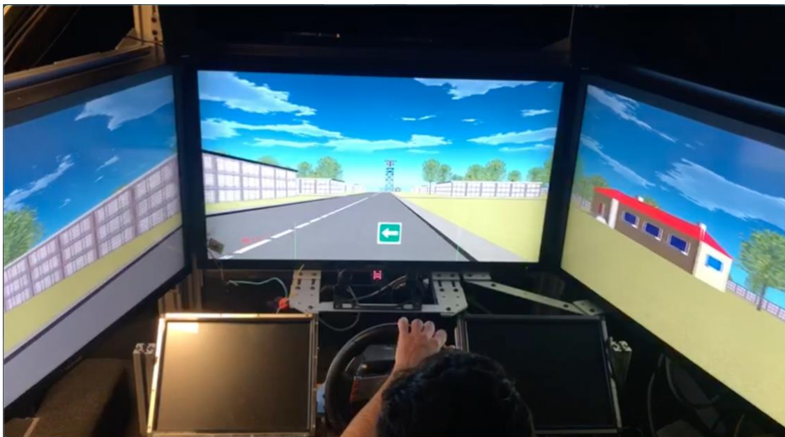
Figure 15: Top: Outside view of the simulator and control interface. Bottom: Inside view of the simulator, showing a participant driving in the virtual town. A colorful house on the right and a radar tower at the end of the street are, respectively, proximal and distal landmarks.
