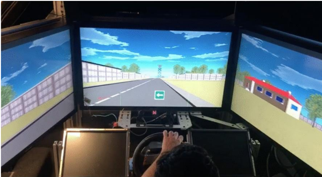
Figure 1: Driving simulator from the participant's view as they completed the guided navigation phase of the combined landmark group (PD group). Participants controlled their vehicle with a steering wheel, gas, and brake pedals. The small screens on the left and right of the steering wheel were not used in this experiment. In this example, a tall radar tower at the edge of the town (distal landmark), and a colorful house at the upcoming intersection (proximal landmark) are visible to the driver. A white/green navigation arrow briefly presented at the bottom of the central screen indicates a left turn at the next intersection.
