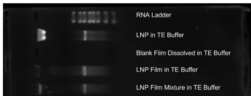
Figure 40: Agarose gel electrophoresis performed on Acuitas-LNPs in buffer, in a film mixture, and in an OTF.
