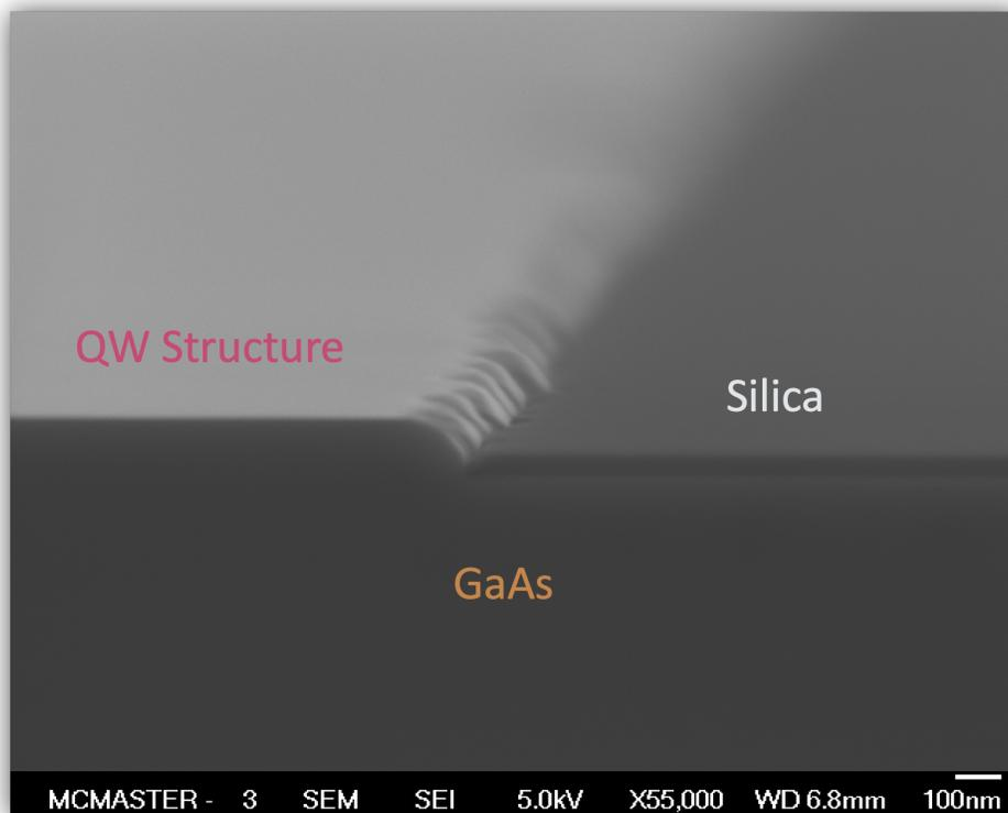
Figure 59: SEM of the InGaAs/GaAs quantum well structure.
