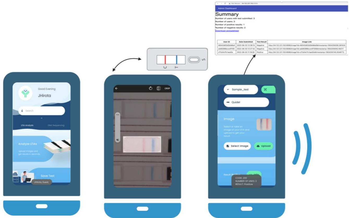
Figure 1.3. VisuFlow©: An open-source cloud framework for smartphone-based LFA diagnostics – improving the interpretation and documentation of LFA results. Front-end user interface (client end) for smartphone application and validation of the sensitivity/specificity and backend admin dashboard. Development of VisuFlow was completed by Manjot Hunjan and Alex Wu.
