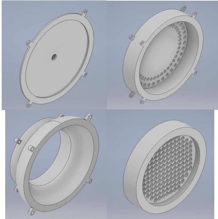
Figure 16. Four 3-d printed parts comprising the diffuser nozzle, top left: Inlet, top right: baffle plate, bottom left: smooth contraction, and bottom right: outlet and flow straightener
