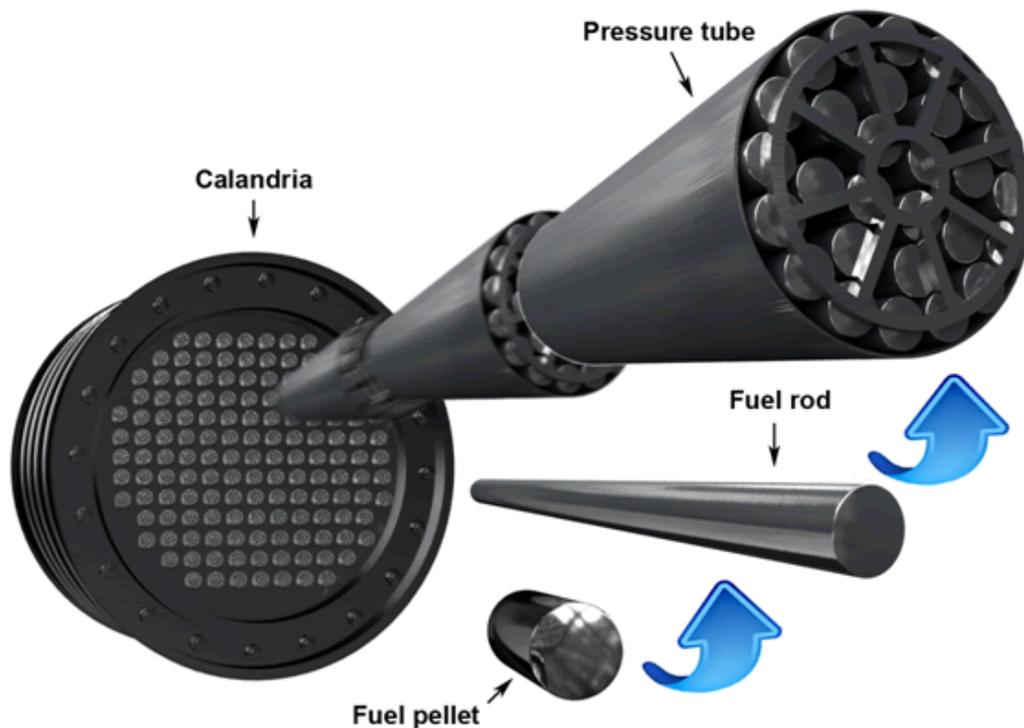
Figure 1. Calandria and pressure tubes of a typical CANDU reactor from [1]
