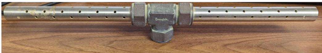
Figure 46. Assembled inlet manifold for section 4 tests
