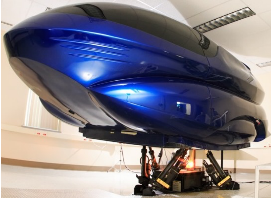
Figure 1. A motion simulator that provided physical- and visual-motion stimuli for the research conducted for this doctoral thesis. The simulator is composed of an enclosed cabin equipped to provide an immersive virtual environment. The cabin is supported by a MOOG © Stewart platform with capability of six-degrees-of-freedom motion.
