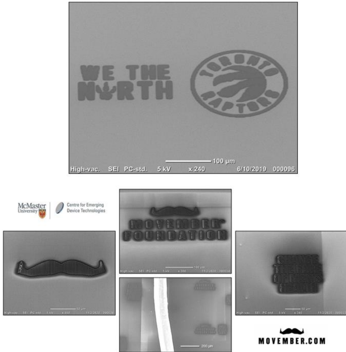
Figure 4.5. Photoresist on Si for promotional samples created using the UV writing process.
