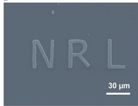
Figure 2.35: Top: Single-shot pattern deposition in LIFT. Bottom: SEM image of deposited pattern [34]. – Permission requested from the publisher.
