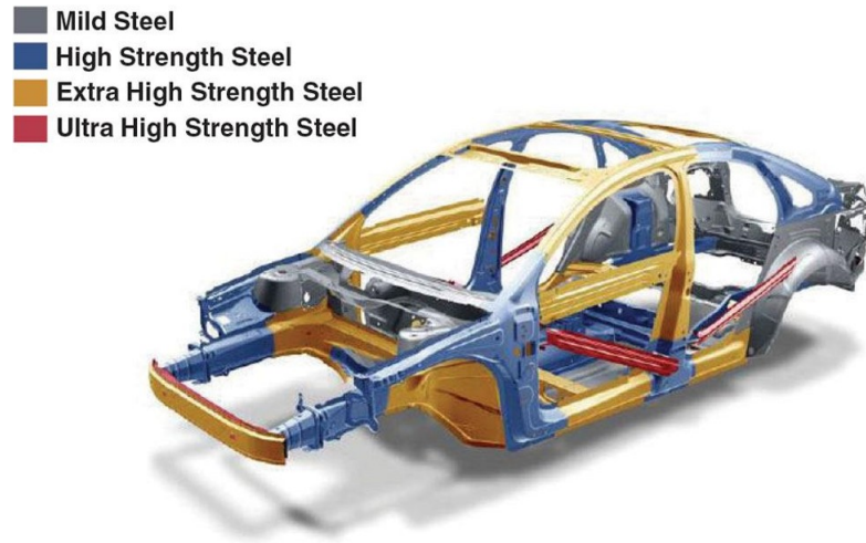
Figure 1.2: Mild steel (grey) and AHSS grades' (blue, yellow, red) distribution in a typical automotive vehicle [8].
