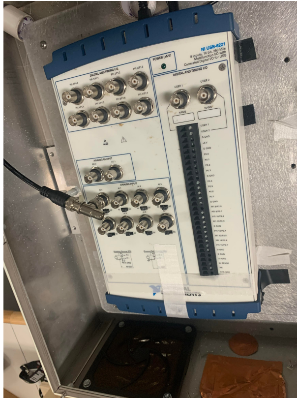
FIGURE 5.7: National Instruments USB-6221 Analog to Digital Converter: Convert analog output from amplifier into 16-bit digital signal computer logging.
