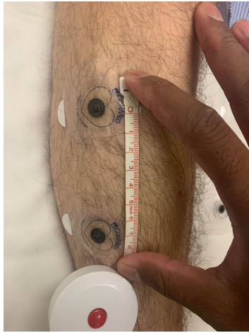
(A) Spacing between readout electrodes: Electrodes placed 7cm apart from edge to edge, distance maintained across all subjects.
