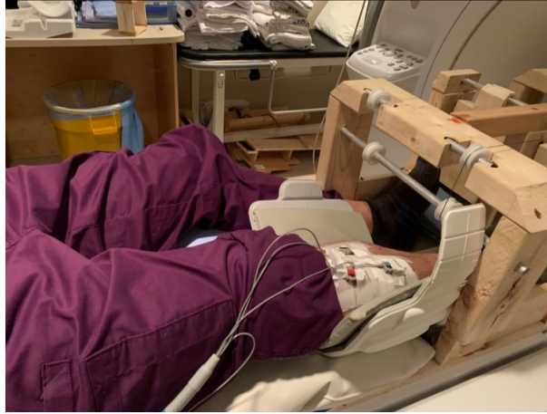
FIGURE 5.24: Subject Leg While Attaching Electrode Leads: Electrodes connected to leads with tape restraining movement of connections. Flex coil padded to distance leg slightly from coil surface. Leg propped up with padding to properly position leg within the lab designed MRI compatible ergometer. Ergometer has been loaded with weight corresponding to subject's 40% MVC.
