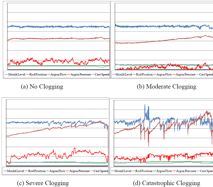
Figure 2-16. Various degrees of clogging in industry (Cathcart, 2018).
