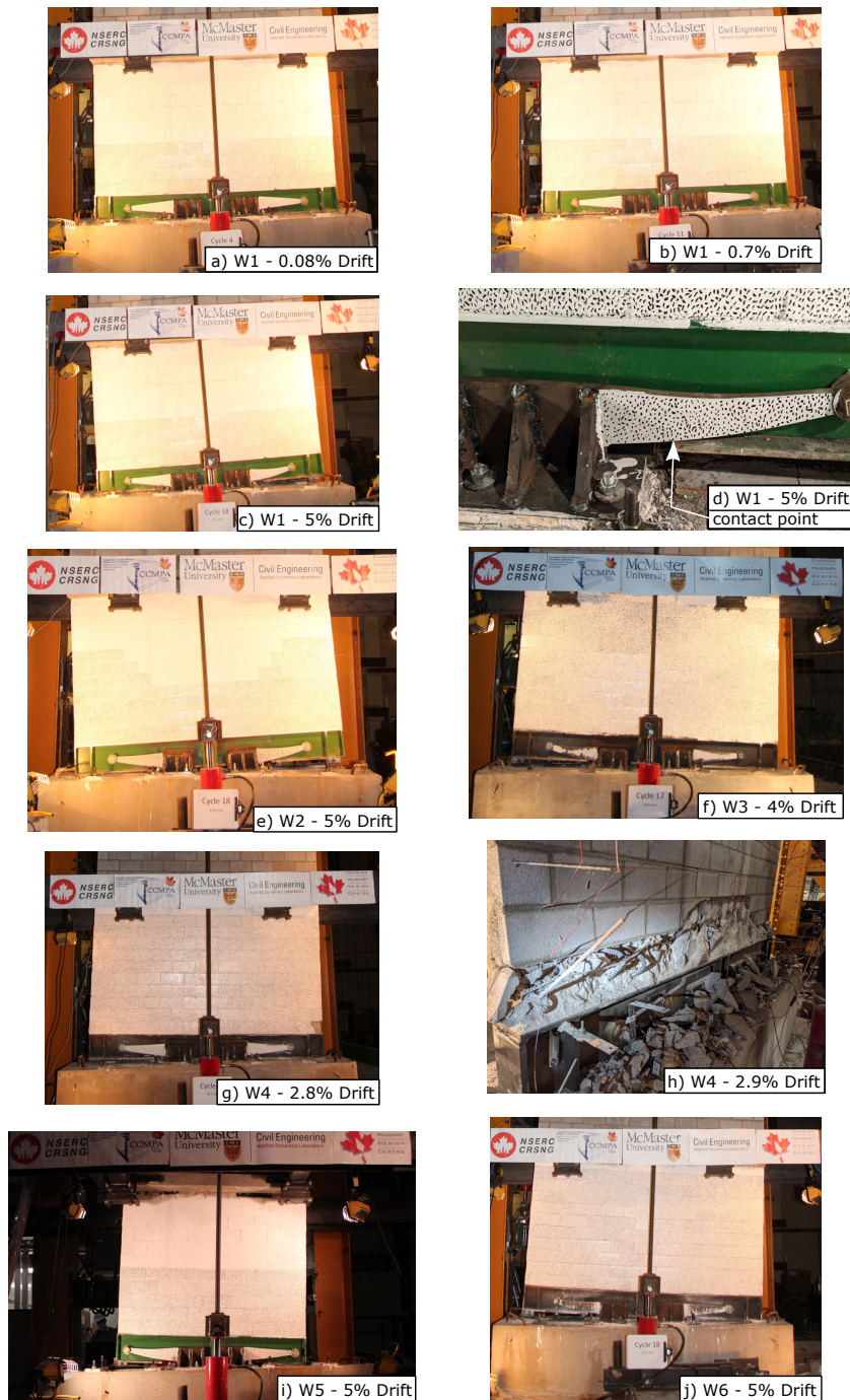
Figure 4.7: Test photos at various drift ratios; a) Wall 1 uplift; b) Wall 1 flexural arm yield; c) Wall 1 peak drift ratio (5% or 125 mm); d) Wall 1 flexural arm contact with steel base at peak drift ratio; e) Wall 2 peak drift ratio; f) Wall 3 peak drift ratio; g) Wall 4 prior to failure; h) Wall 4 post-failure; i) Wall 5 peak drift ratio; and j) Wall 6 peak drift ratio
