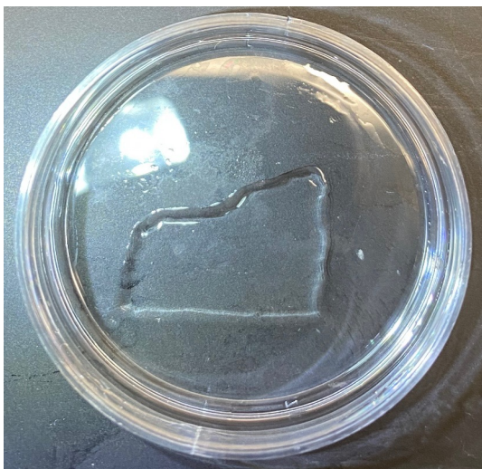
Figure 14: Example of a fully expanded LSO gel in a petri dish after the removal of ddH 2 O.
